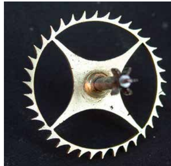
Figure 3 (top). Warn wheel with a parallel arbor and a brass collet.
