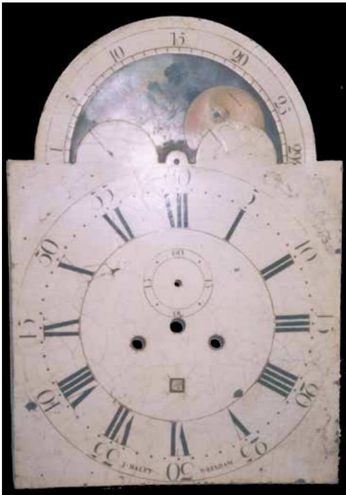
Figure 6. One of the earliest Birmingham painted dials, made for J Haley of Wrexham, with a calendar ring, but no falseplate. The crazing due to the top layers 'floating' on the bituminous base layer is not visible in this image. Photograph J Robey.
