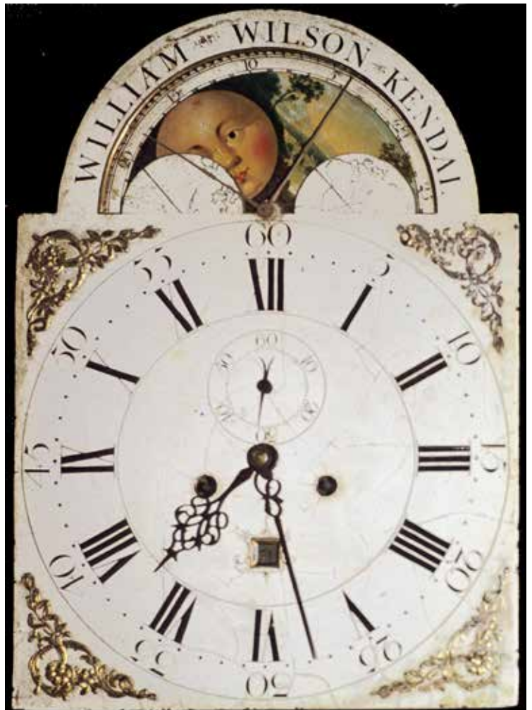
Figure 7. Painted dial made for William Wilson of Kendal (not related to James Wilson) in a case dated 1774. Repoussé brass spandrels, silvered date ring, early half hemisphere maps, and no brass collets round the winding holes. The moon has a small track of Roman numerals with two pointers to indicate high tide at two different ports. Photograph J Betts.
