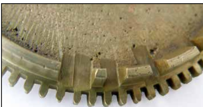
Figure 12 (top). The slots cut into a hoop cast integral with the wheel.
