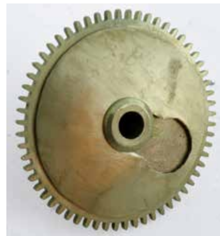
Figure 10. The slip washer holds the hour wheel on its pipe.
