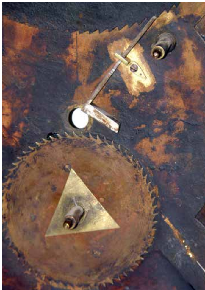
Figure 14. The rear of the dial showing part of the moon dial, the pusher rod and the calendar.
