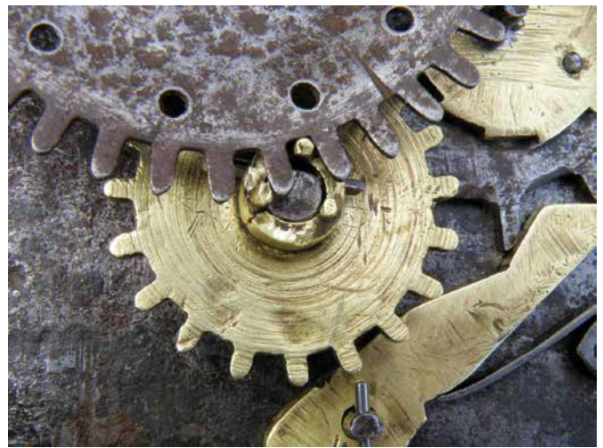
Figure 9. The pinion-of-report meshes very deeply with the hour-wheel teeth.
