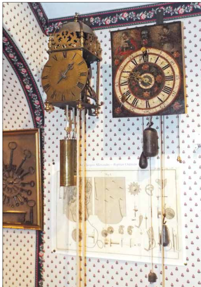
Figure 18. The German silent-pull timepiece alongside a French rack striking lantern clock (see 'French Lantern Clock with Rack Striking', HJ, May 2016, pp222-8).
