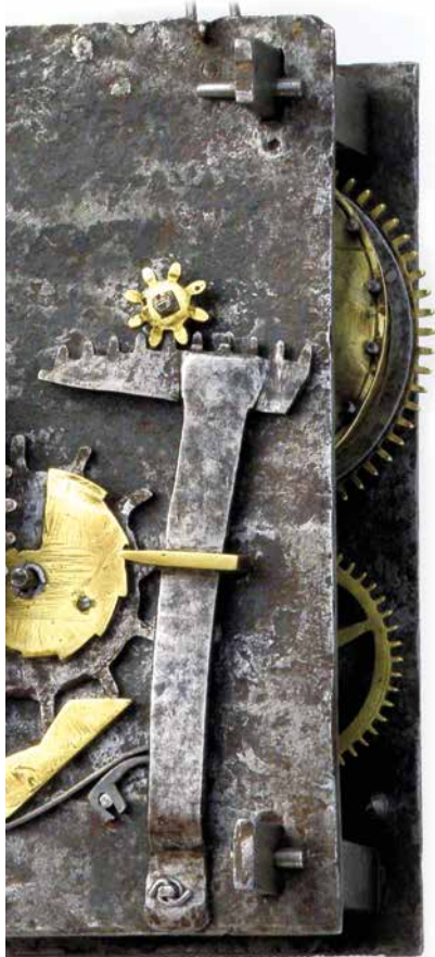
Figure 12. The rack driven by a brass pinion on the barrel arbor.
