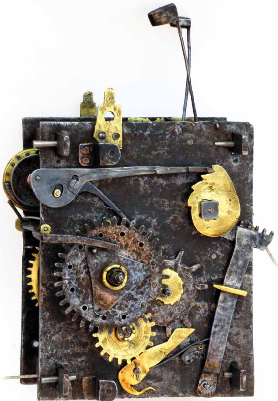
Figure 13. Front of the movement with the silent pull locked.
