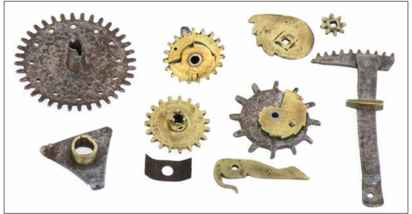
Figure 8. The motion-work (left), quarter locking cam, pinion, rack, starwheel with hour snail and jumper (right).
