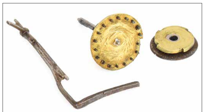
Figure 6. Alarm release lever, crown wheel with pins and weight pulley.
