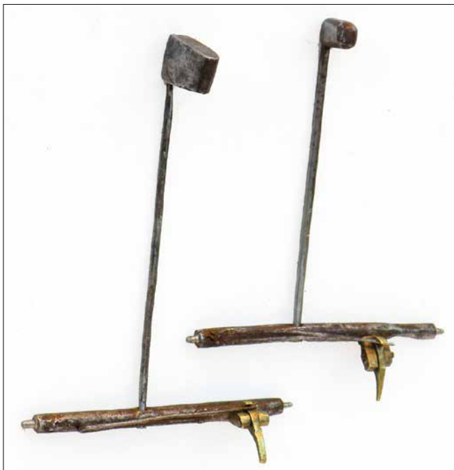
Figure 15. Hour and quarter hammers with pivoted tails and biasing springs.
