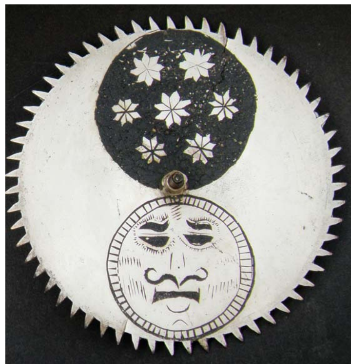
4. The moon disc has a full moon and a 'dark of the moon', with 59 teeth round the edge.
