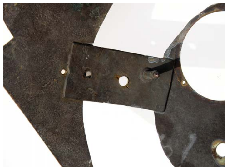
6. One of the four straps holding the dial centre to the outer part.
