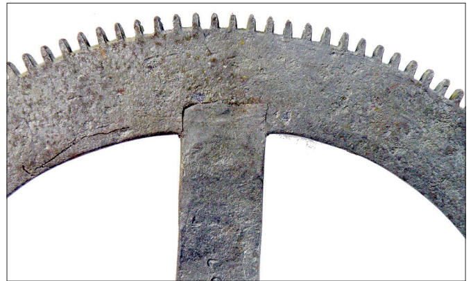
Figure 17. Greatwheel of a French iron clock, about 1580-90, with wide crossings the same thickness as the rim.
