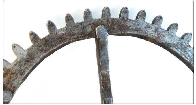
Figure 16. The going greatwheel with thick narrow crossings, typical of Germanic clocks. Note the punch marks made on the tips of the teeth during dividing.
