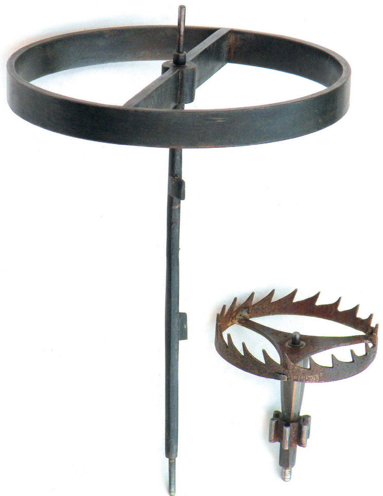
Figure 14. The new balance, crownwheel and pinion.
