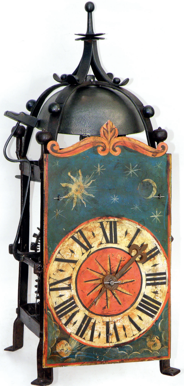
Figure 23. The completed restoration with a new dial and iron hand.
