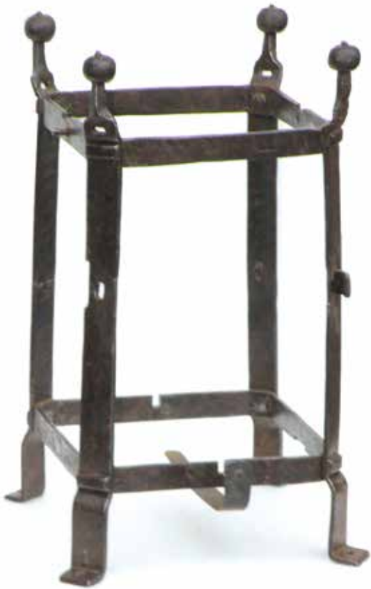
Figure 5. The riveted frame with the later supports for the warning arbor removed and the hammer spring reinstated. Note the holes for the ends of the bell frame.
