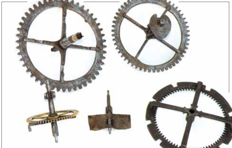
Figure 10. Striking train as found. Clockwise from top left: greatwheel, second wheel with single 'heart' overlift cam, countwheel with internal teeth, later fly, third arbor with locking arm and added brass warning wheel. Note the wear on the crossings of the greatwheel caused by the winding click.
