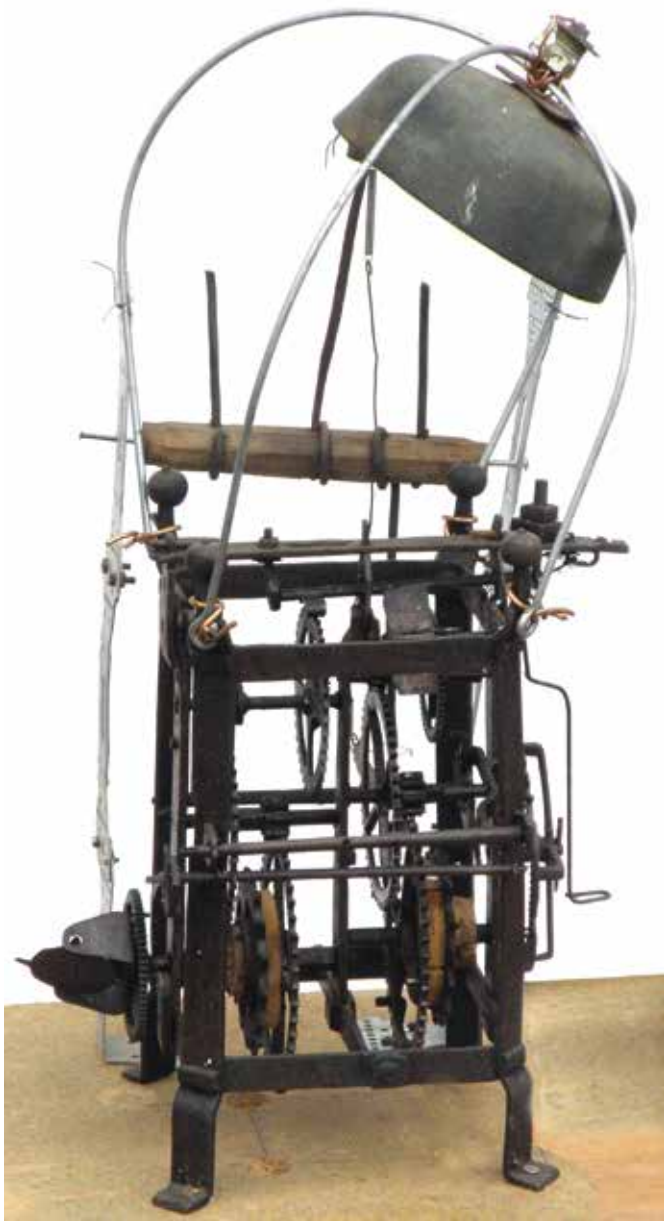
Figure 3. Movement as received with crude additions to use it as a small turret clock.
