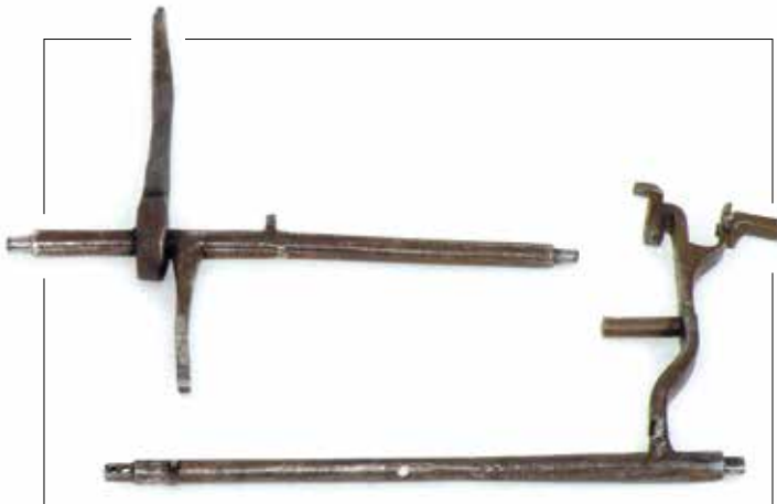
Figure 11. The strike-work as received, top: hammer arbor; bottom: arbor with striking detents, an added link and hole where the lifting piece with nag's head once fitted.
