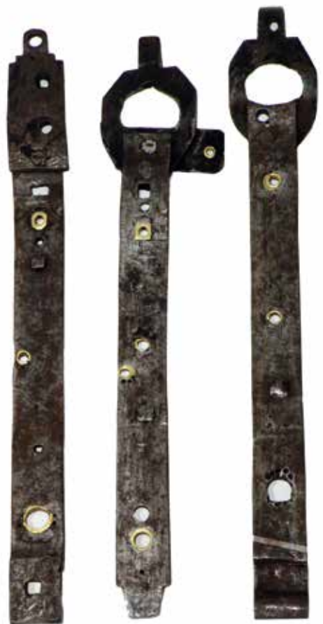
Figure 6. The movement bars with extensions riveted to the top when converted to anchor escapement and one on the central bar for an internal fly. The brass bushes are repairs. Note the holes where supports for the dial, and cocks for the crownwheel and balance were originally fitted.
