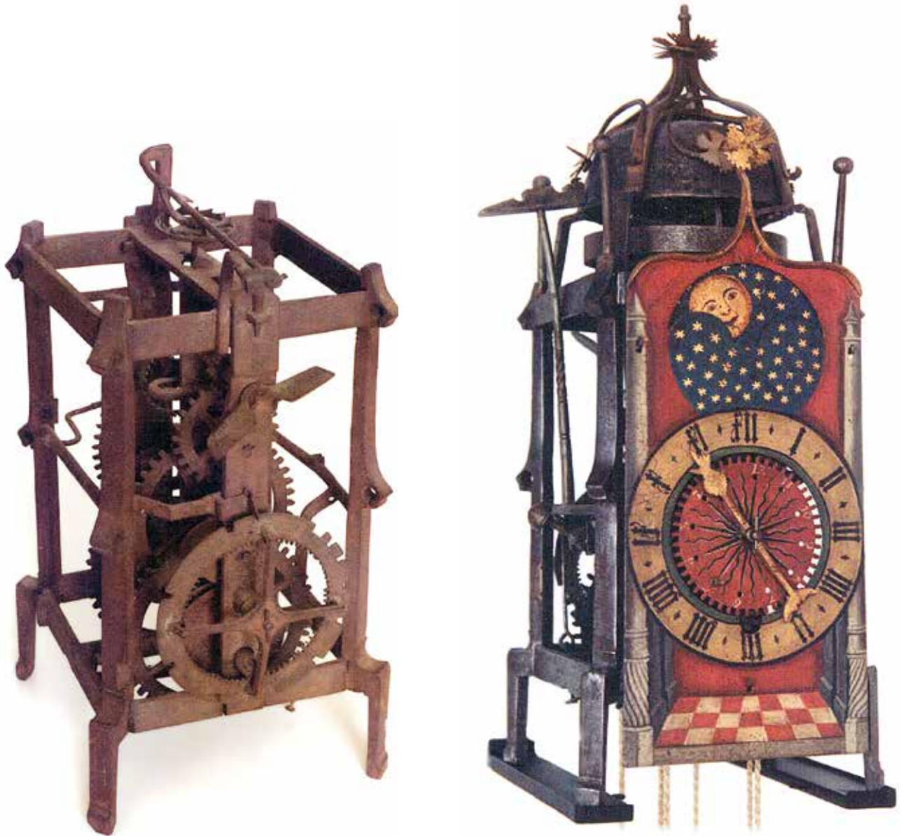
Figures 1 and 2. An early Gothic clock before and after 'restoration'. The escapement, balance, hour wheel, dial, hand, linials, hammer, bell and bell frame are all new. (Photos: Derek Pratt)
