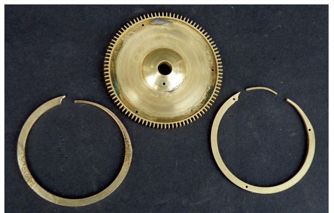
Figure 16. The fusee wheel after removal of the broken spring (right) and the new one (left) ready for fitting.
