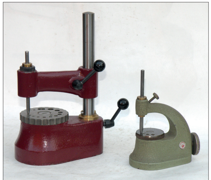
Figure 11. A watchmaker's staking tool (right) and the larger versatile JMW staking tool (left).
