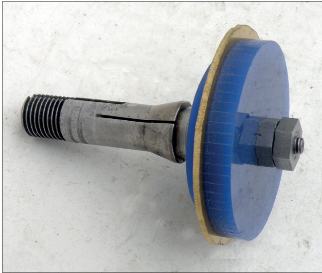
Figure 12. Brass disc held between Perspex backing discs in a mandrel made from an old collet.
