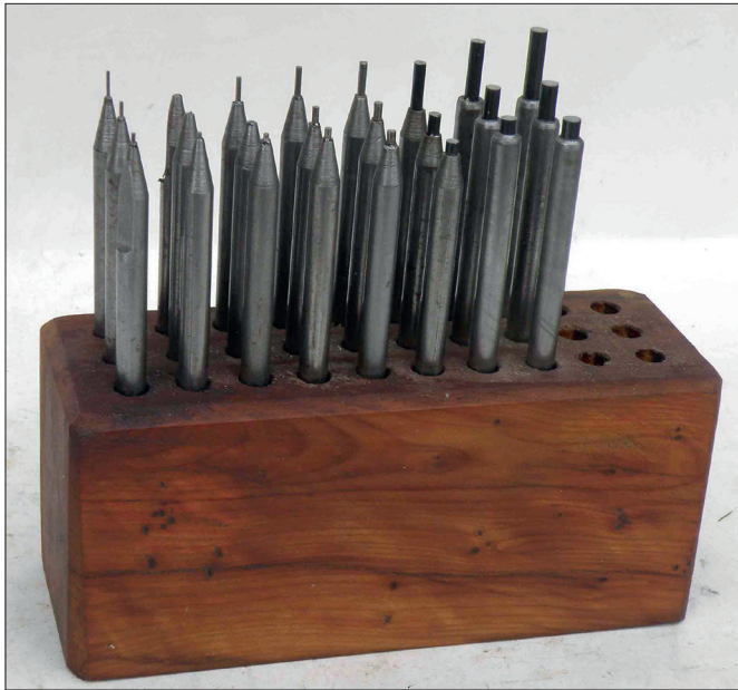
Figure 9. Set of homemade punches with spaces left for additional sizes and a couple awaiting repair.
