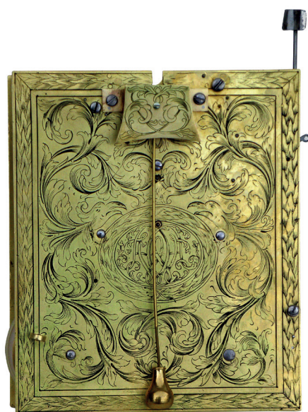
Figure 2. The engraved backplate with a restored verge pendulum and replacement verge end plate.
