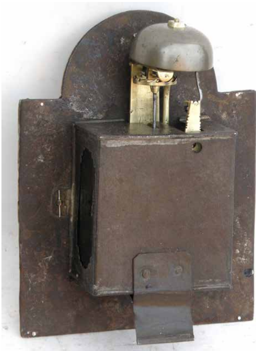
Figure 2. The movement is enclosed in a tinplate box leaving the crownwheel and verge escapement exposed.
