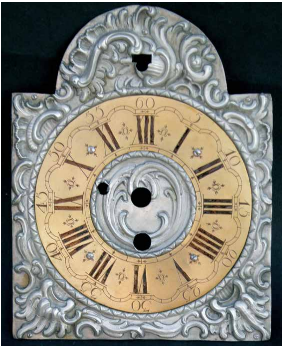
Figure 8 (right). The dial of the bedroom alarm after cleaning and silvering and with the chapter ring re-gilded.
