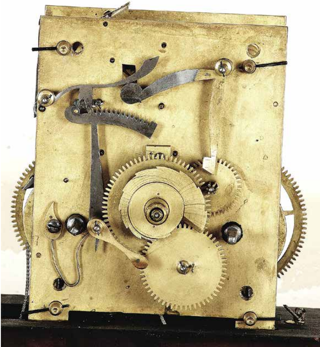
Figure 7. The movement on the Dilger & Barclay clock, standing on short feet and a horizontal hammer to strike on a gong.
