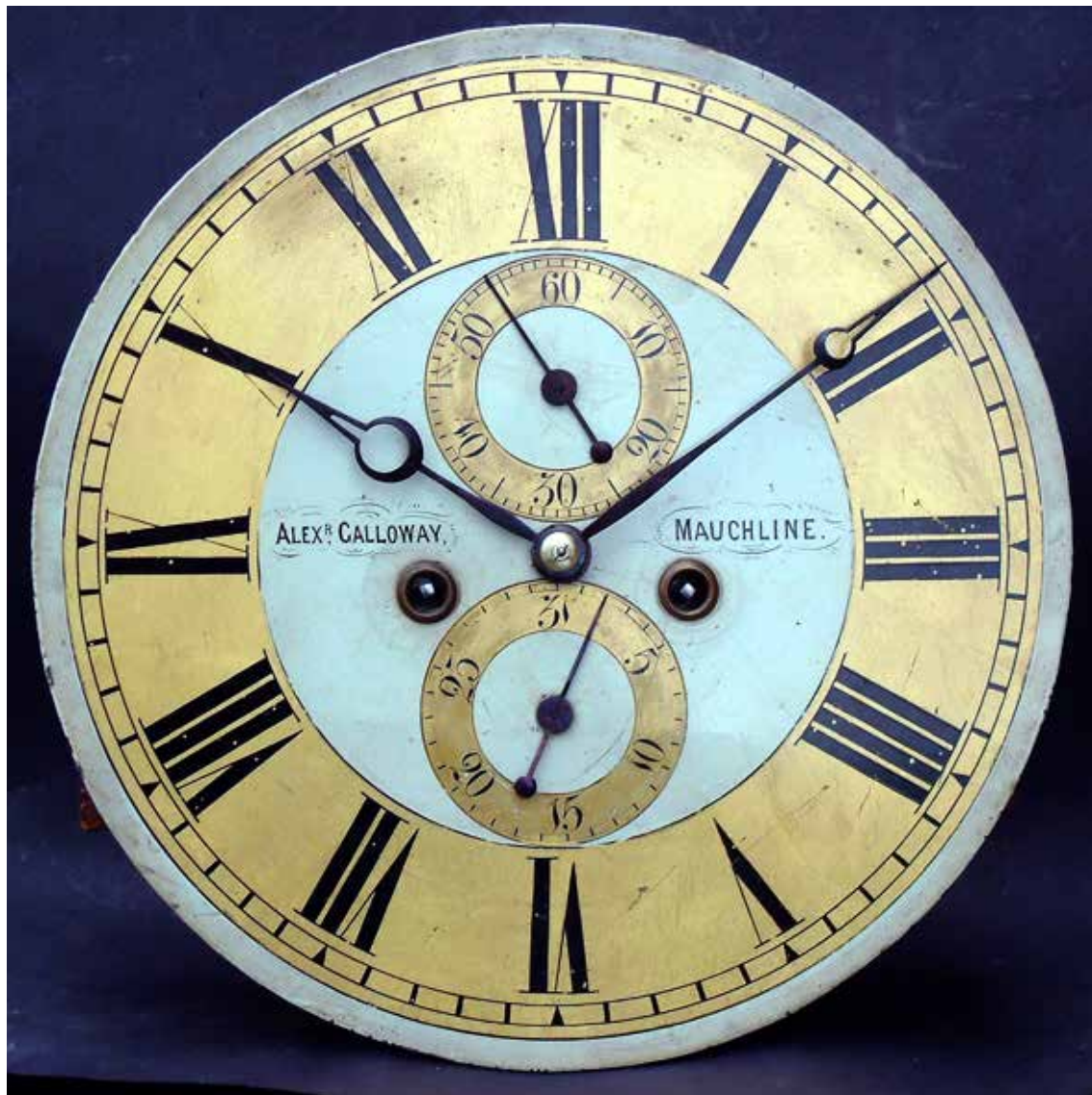
Figure 4. Round iron dial with a white centre and gilt chapter, seconds and calendar rings.
