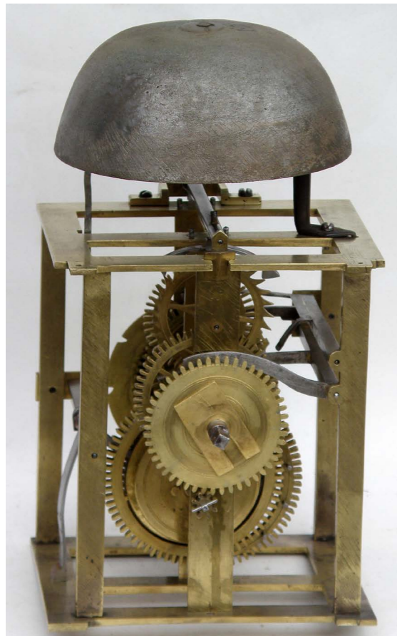
Figure 8. Movement from the front showing the skeletonised frame.
