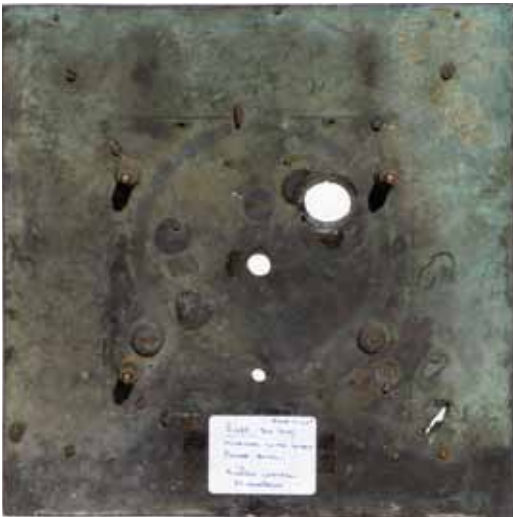
Fig. 2. Dial rear showing the rollers for the missing date ring and the friction 'washers' for the subsidiary indicators. Note the very wide spacing of the dial feet (one missing).
