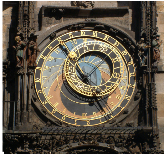
Fig. 8. Astrolabe type of astronomical dial on the clock on the Old Town Hall, Prague, 1410.
