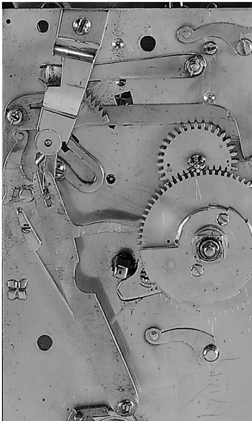
Fig. 16. Detail of the rack striking mechanism. An extension of the vertical lever falls onto the snail, its motion being transferred to the rack via a pin and slot, rather than a rack tail. The rack hook is pivoted on the right and the lifting piece is of the type used with countwheel striking, © Christie's Images Ltd.
