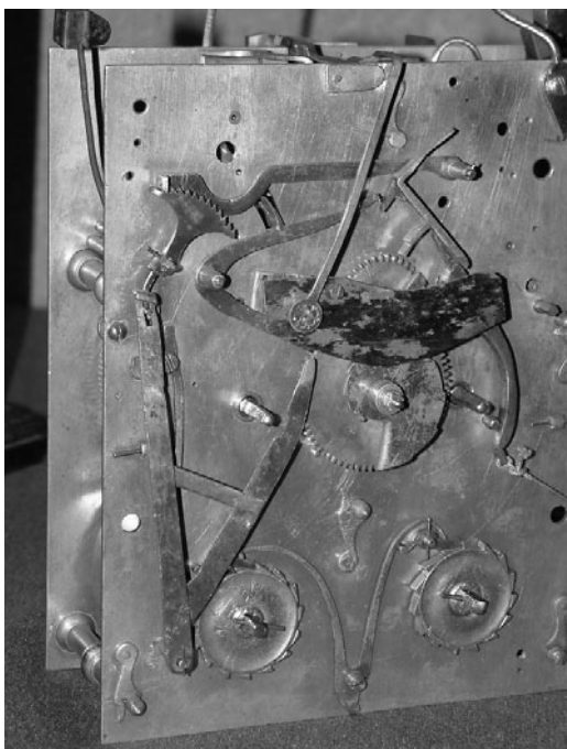
Fig. 11. Front view of the movement, showing the external rack for holding with a rack hook. One arm of the V-shaped lever falls onto the snail, while a slot in the other arm links with a pin on the external rack.
