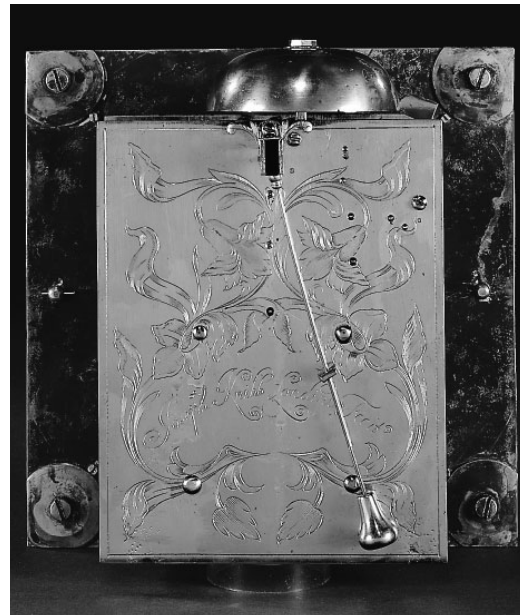
Fig. 14. Backplate of the Knibb clock, with no evidence of an earlier countwheel, © Christie's Images Ltd.
