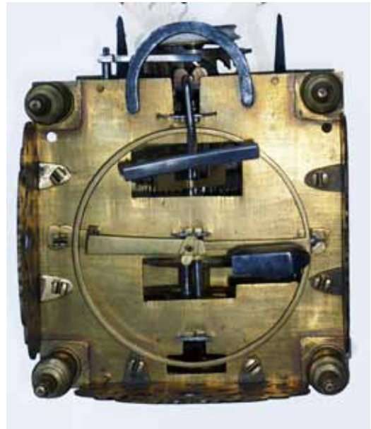
Fig. 9. Unaltered top plate of the Norris clock with its original balance and alarm. (Photo: Brian Loomes)
