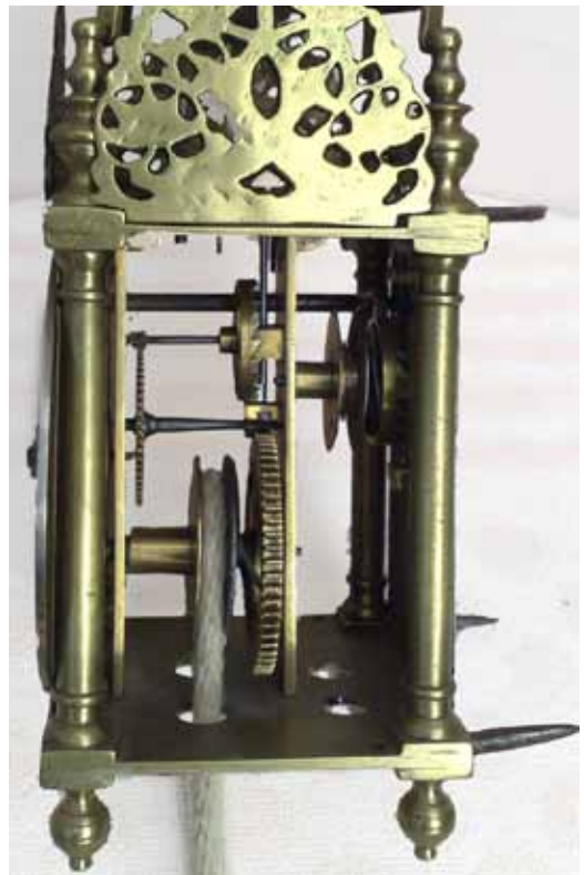
Fig. 44. The escapement of Clock 10. (Photo: Martyn Pettifer)
