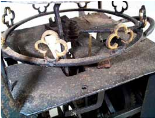
Fig. 36. Detail of the balance of Clock 8 with cast-brass quatrefoil attachments. (Photo: J. Hooper)
