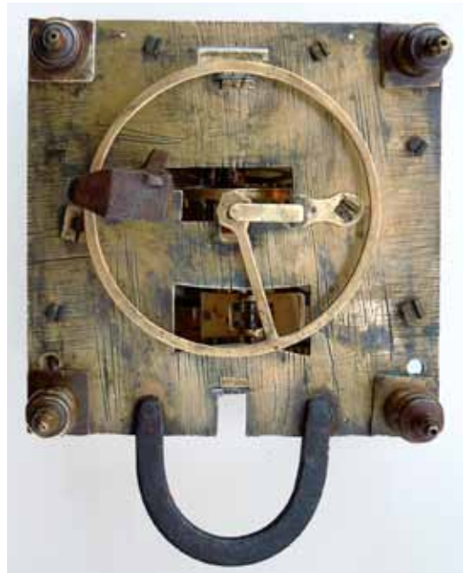
Fig. 27. Samuel Stretch de Leeke with unaltered top plate and balance. The shape of the central boss indicates that the balance was probably cast with four arms to avoid distortion, three of them removed during finishing. (Photo: private collection)
