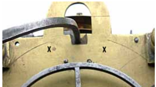
Fig. 2. Reconverted Crockford clock with an incorrect iron balance and a reinstated alarm. There is no aperture for the fly as it is below the top plate, which has an integral hoop. (Photo: private collection)
