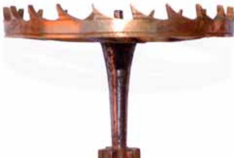
Fig. 34. Stretch de Leeke crownwheel with undercut teeth, and original steeply tapered arbor (Photo: private collection)
