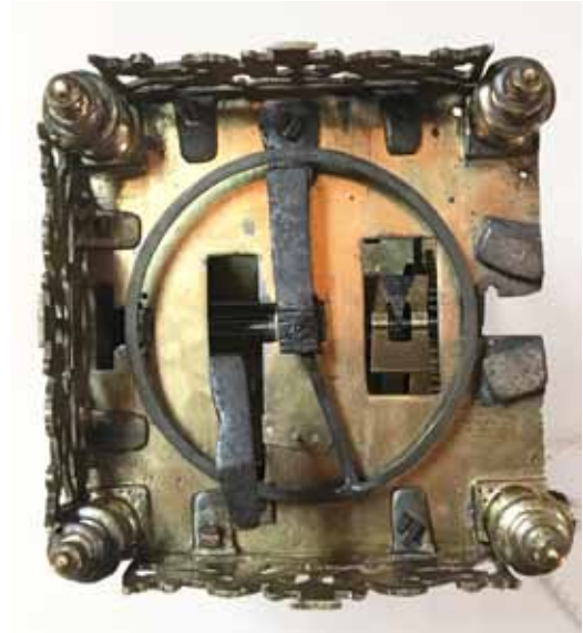
Fig. 12. The tarnished brass balance of the Pennocke clock with an original iron top cock. (Photo: W. F. Bruce, courtesy of J. Nye)
