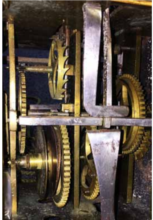
Fig. 54. The Fromanteel crownwheel appears to be a replacement. (Photo: private collection courtesy of Brian Loomes)
