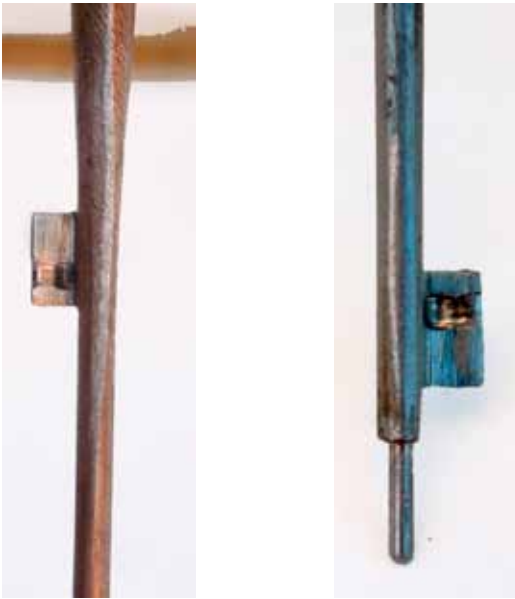
Figs 31-32. Wear on the Stretch de Leeke pallets. Note the shape of the top of the verge. (Photo: private collection)
