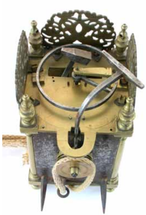
Fig. 2. Reconverted Crockford clock with an incorrect iron balance and a reinstated alarm. There is no aperture for the fly as it is below the top plate, which has an integral hoop. (Photo: private collection)
