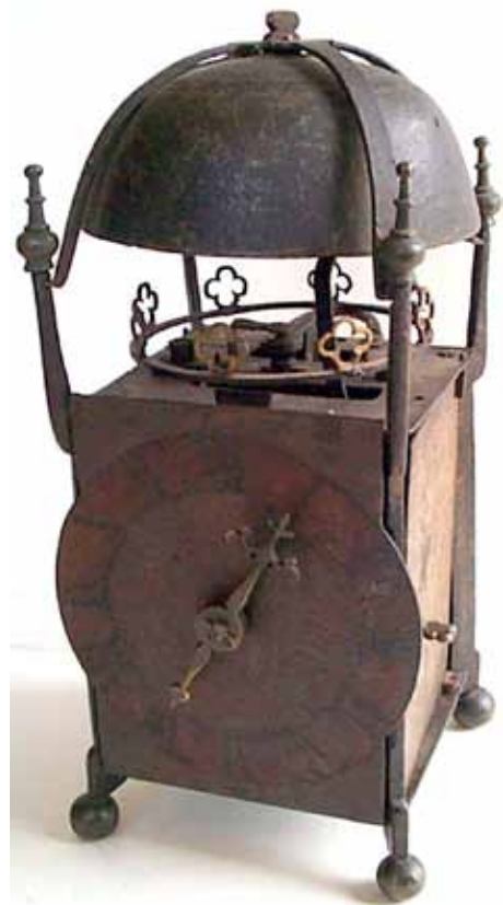
Fig. 35. Clock 8, anonymous English lantern clocks with an iron frame and balance. (Photo: J. Hooper)
