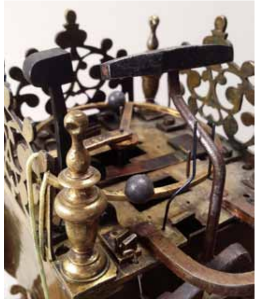
Fig. 15. Unaltered top plate of the Prime clock. The original balance has two lead balls, one original, the other a replica. (Photo: B. Calver)
