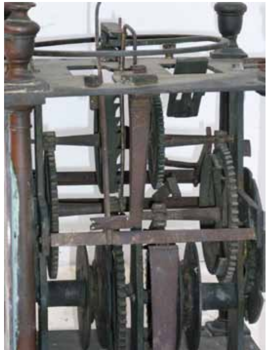
Fig. 19. Original balance and escapement of the Quelch clock. (Photo: Brian Loomes)
