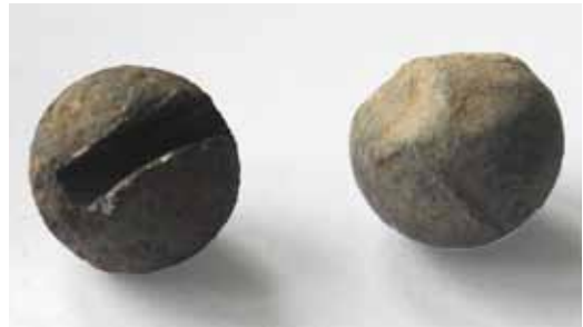
Fig. 16. The original Prime slotted balance weight (left) compared to a Civil War musket ball (right). (Photo: B. Calver)
