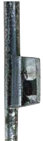
Fig. 23 (right). Lower pallet of Stretch clock, with two wear pits.
