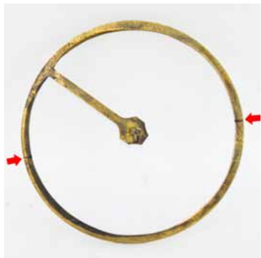
Fig. 28 Underside of the original Stretch de Leeke balance with the inner edge partly chamfered for poise. The arrows indicate the position of the marks shown in Figs 29-30. (Photo: private collection)
