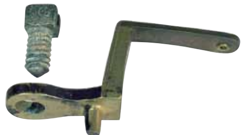
Fig. 25 (below) . Balance top-cock of the Stretch clock, with an integral cast steady pin, and an original fixing screw. (Photos: J. Darken)
