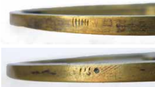
Figs 29-30. File marks on the Stretch de Leeke balance indicate the former position of lead weights. What appears to be a punch mark is a small casting fault. (Photo: private collection)
