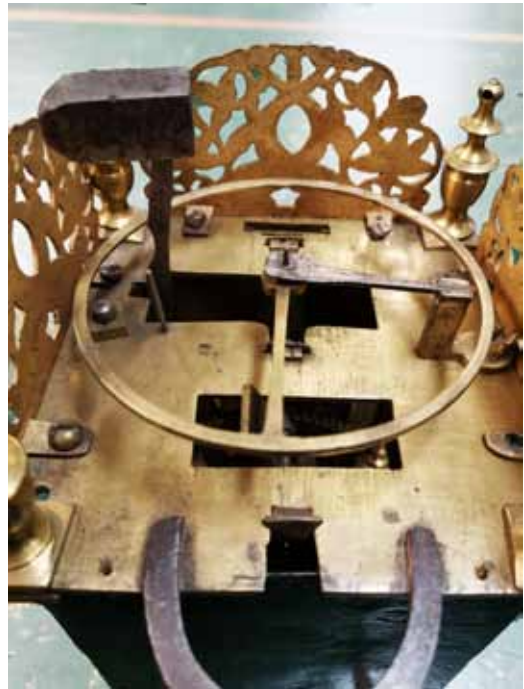
Fig. 6. Clock 1, top view showing the balance and repaired top cock. (© Trustees of the British Museum)
