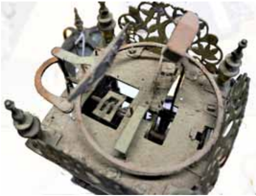
Fig 49. Unaltered top plate and alarm of the Closon clock, though the iron balance is probably later. (Photo: private collection courtesy of Brian Loomes)
