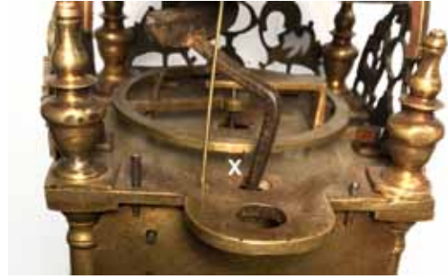
Fig. 40. The balance of Clock 9 with one of the plugged holes in the side of the rim marked by X. (Photo: Nigel Raffety)
