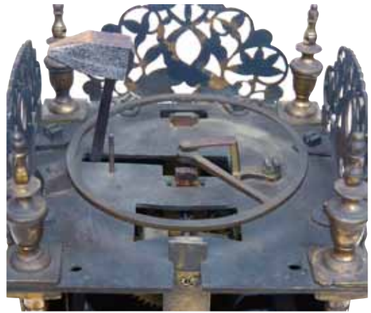
Fig. 21. Unaltered top plate and balance of the Stretch clock. Hanging hoop missing. (Photo: J. Darken)
