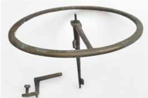
Fig. 53. The Fromanteel balance with rounded edges appears to be original, but the verge is overly sturdy with little pallet wear. (Photo: private collection courtesy of Brian Loomes)
