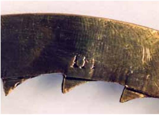
Fig. 1. IM casting mark on the calendar ring of an 8-day longcase clock signed for Simon Thorn, Tiverton, Devon, about 1740. This mark is also on the hour wheel. Both the dial and the five-pillar movement were probably supplied from London.
