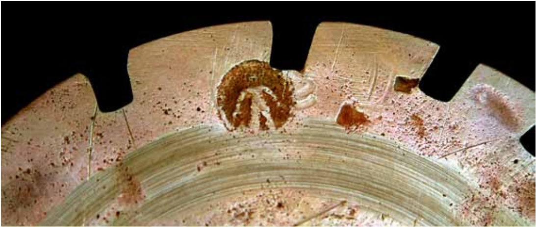
Fig. 15. 'Matchstick man' casting mark on the countwheel of a lantern clock by Peter Closon, about 1650.
