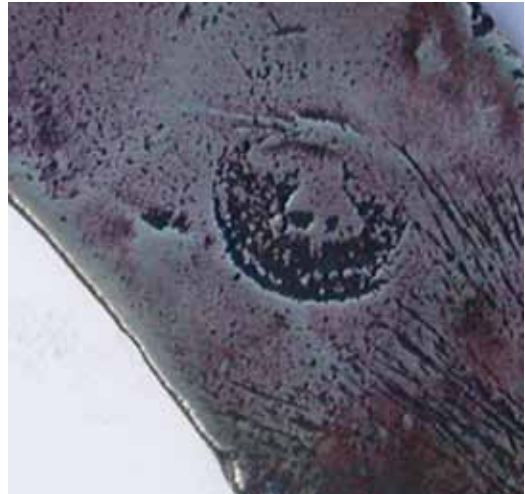
Fig. 17. Bell casting mark on the rear of the chapter ring of an unsigned Lothbury lantern clock of the 1650s, possibly by Thomas Loomes. (Photo: Brian Loomes)
