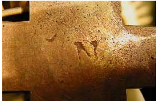
Fig. 11. N casting mark on all three movement bars and the chapter ring of a posted-frame 30-hour clock by John Bronson, Stowmarket, Suffolk, about 1740. (Photo: R. Fryatt)
