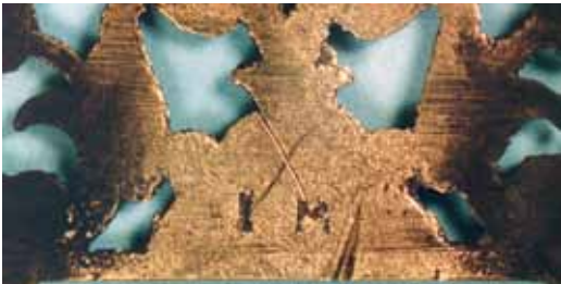
Figs 4-6. Components of a miniature lantern alarm by John Rogers, Leominster, Herefordshire, about 1760, with casting marks: M on the crownwheel and alarm disc, and IM on the rear of the fret.
