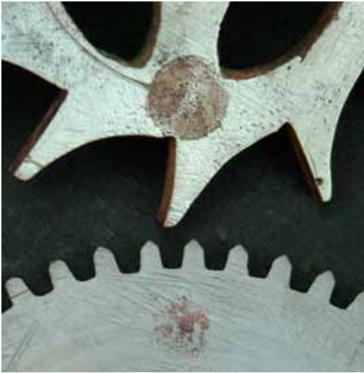
Fig. 16. Less clearly defined marks on the starwheel ('ratch') and hour wheel of the same Closon lantern clock.
