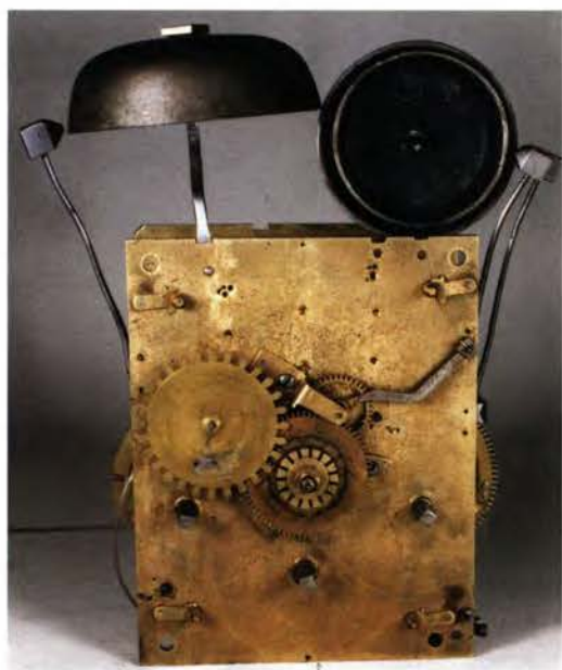
Fig. 5. Front of the Taylor three-train movement. Note how the incorrectly divided 12-hour wheel has been corrected by using pins to drive the 24-hour calendar wheel. The bells were planned to be on the opposite plates to their current location.
