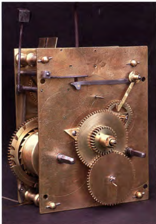
Fig. 22. Sandiford's movement has countwheel striking with the type of lifting/warning piece that was used on racking clocks.
