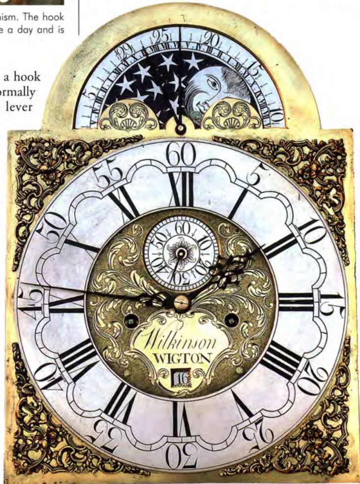
Fig. 16. Dial by Joseph Wilkinson of Wigton, about 1760, with a rolling moon in the arch also indicating the times of high tide at two ports.
