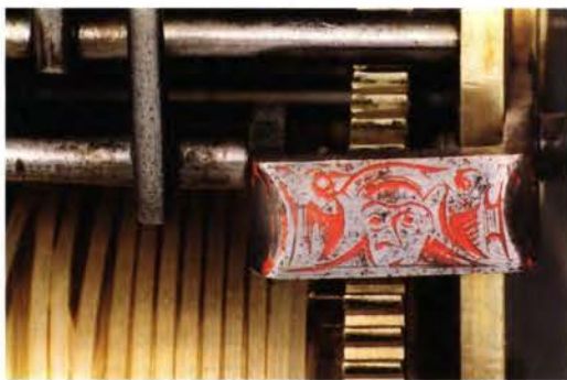
Fig. 8. The lower ting-tang hammer arbor is supported on an iron bracket to clear the great wheel and is engraved with a face.
