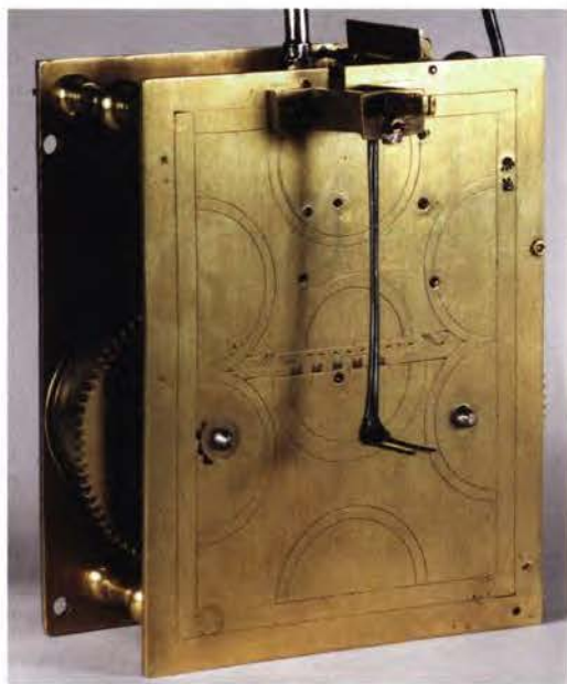
Fig. 13. The rear plate is engraved with decorative lines and semicircles.
