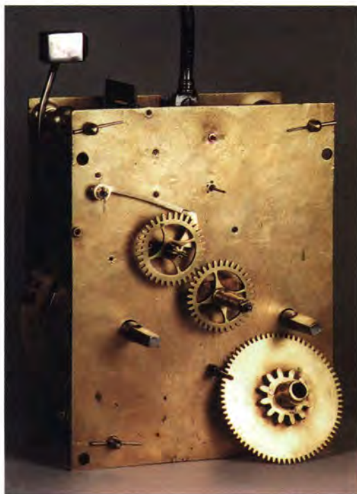
Fig. 11. The Bancroft movement has no bridge for the hour wheel.
