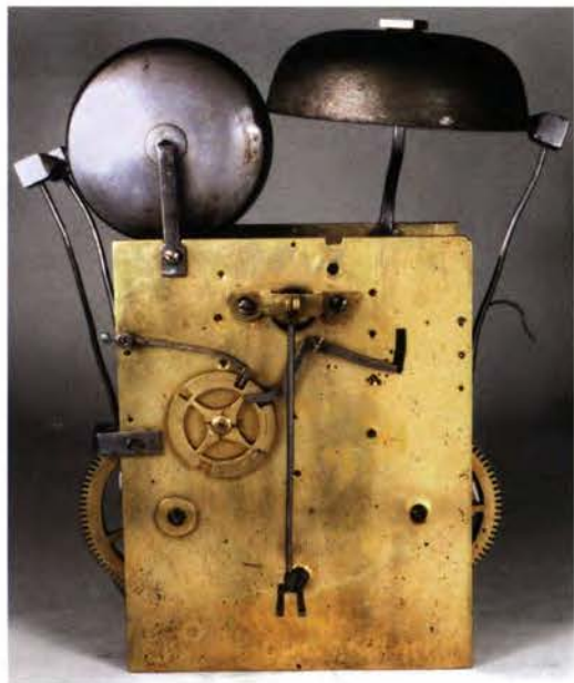
Fig. 6. Movement rear showing the pin on the small external quarter countwheel that trips a pivoted lever to unlock the hour strike. There is no warning before the hour.
