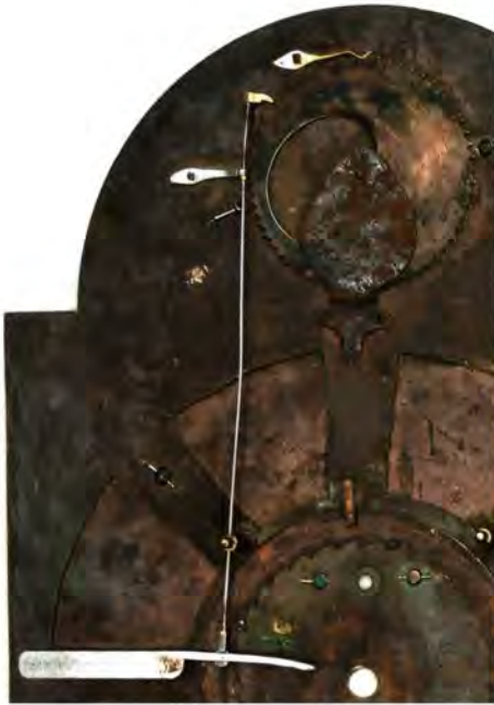
Fig. 15. Restored moon operating mechanism. The hook on the end of a wire pulls the moon twice a day and is returned by a counterweight.
