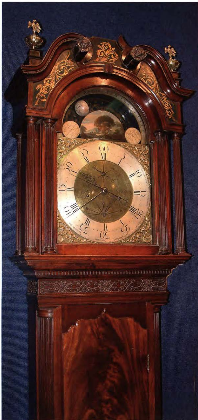
Fig 41. Astronomical clock by Barry of Leigh in a mahogany Liverpool case. The globe moon rotates on its axis and also moves across the arch once a day.
