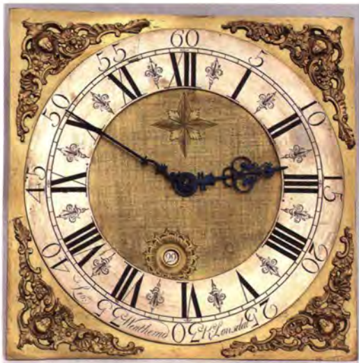
Fig. 28. Thirty-hour dial by Leonard Weatherhead, Kirkby Lonsdale with an off-centre vertical calendar. Course matting done vertically and horizontally. Restored hands of a pattern used by this maker.
