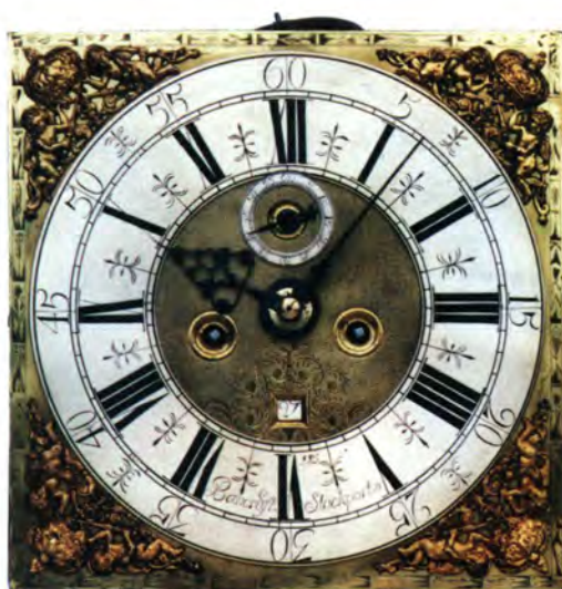
Fig. 10. Dial signed 'Bancroft Stockport' and numbered 115. Note the slip washer for setting the hour hand in front of the hand rather than behind the hour wheel.
