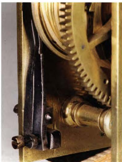
Fig. 7. The Taylor movement has adjustable tension for both the two ting-tang hammers (seen here) and the hour hammer.
