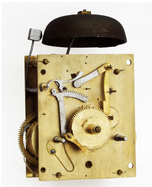
Fig. 8. Typical characteristic Harlow rack-striking eight-day longcase movement, supplied to a Bedfordshire retailer in 1802. It is identical to the engravings in Samuel Harlow's The Clock Makers' Guide .
