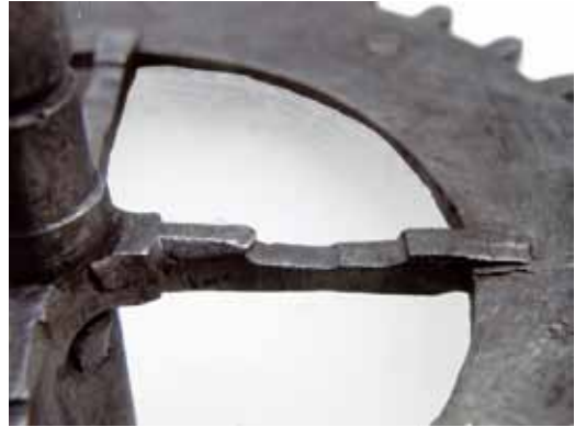
Fig. 12. The crossings of both greatwheels have two sets of wear from previous spring clicks.
