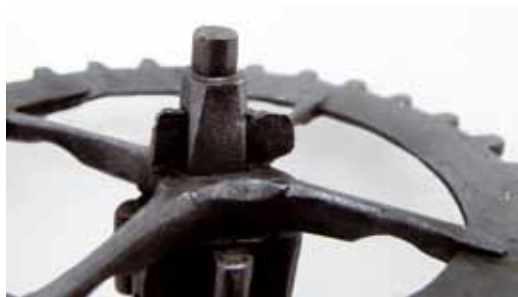
Fig. 8. Second wheel of the striking train fixed to its arbor by a wedge. Sections of each crossing are reduced in thickness to give clearance for the hammer pins.
