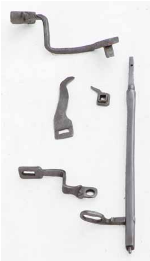
Fig. 15. The vertical hammer shaft. The hammer head and a small arm for the spring fit on a square, while the top support and stop both fit on a lug on the top of the frame and are held by a wedge.
