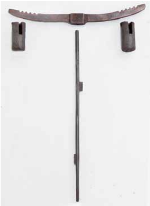
Fig. 17. Replica verge with removable foliot.
