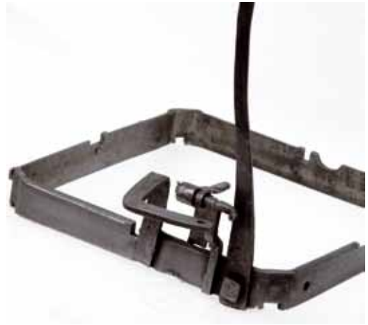
Fig. 16. The lower sub-frame with the vertical hammer spring, hammer tail and the later hammer support.
