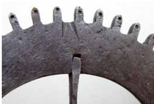
Fig. 9. Punched dots on the teeth of the going greatwheel. Note the mark for correct engagement with the pinion of the second wheel.
