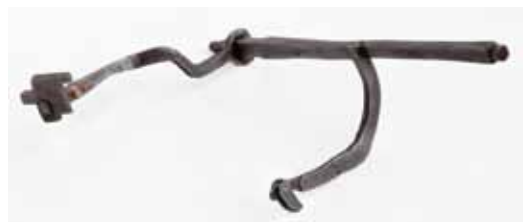
Fig. 14. Arbor for the strikework, with a nag's head in the middle and a combined locking, overlift and countwheel detent at the rear.
