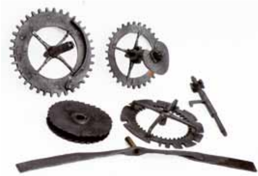
Fig. 11. The two-wheel striking train with rope pulley, countwheel, fly/locking arbor and external fly.
