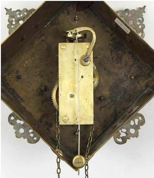
Fig. 2. The original verge escapement. (Photo: F. Ballestrem)
