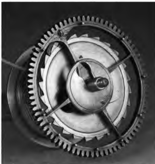
Fig. 2. Internal pin countwheel on an 8-day longcase clock by John Haywood of Northwich, about 1790-1800.
