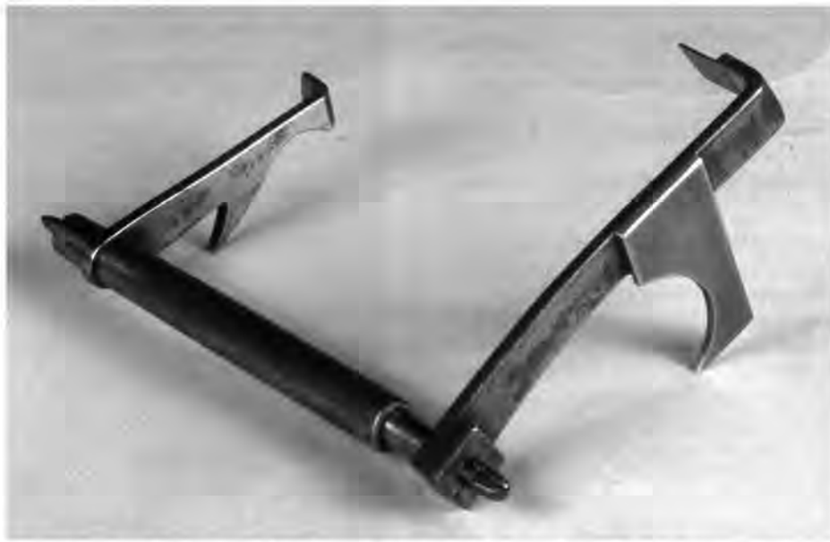
Fig. 3. Single striking arbor of the Haywood clock, with just two levers. The front one has a brass lifting piece and the warning detent; the rear lever has the locking detent and countwheel detent.
