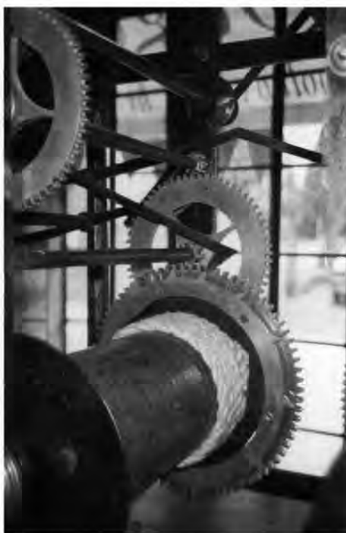
Fig. 1. Turret clock made by William Stumbels of Totnes for Dartington Hall in 1741, with the striking controlled by raised projections on the countwheel.
