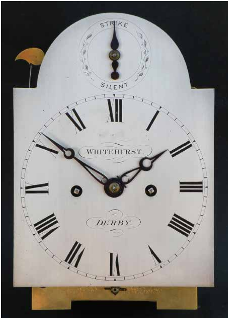
Figure 2. The single-sheet silvered brass dial.
