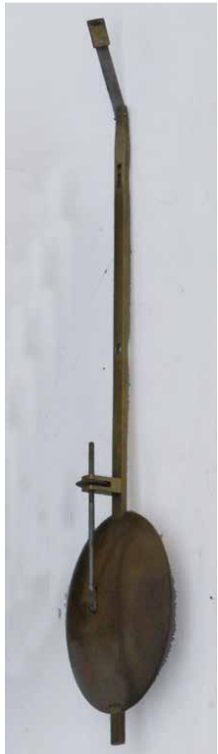
Figure 9. Pendulum adjustment above the bob on a chiming bracket clock by Brockbank & Atkins, London.
