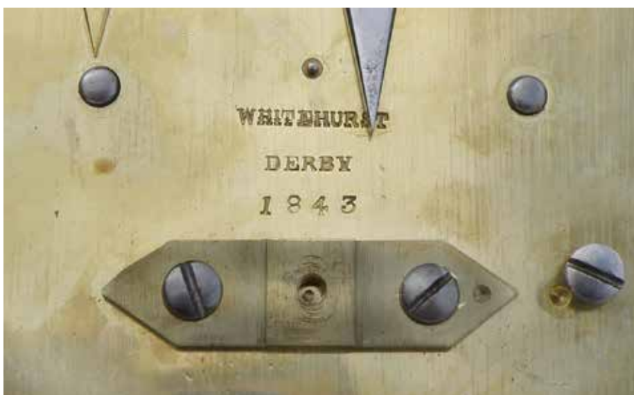
Figure 5. The hold-fast for the pendulum, stamped name and date.
