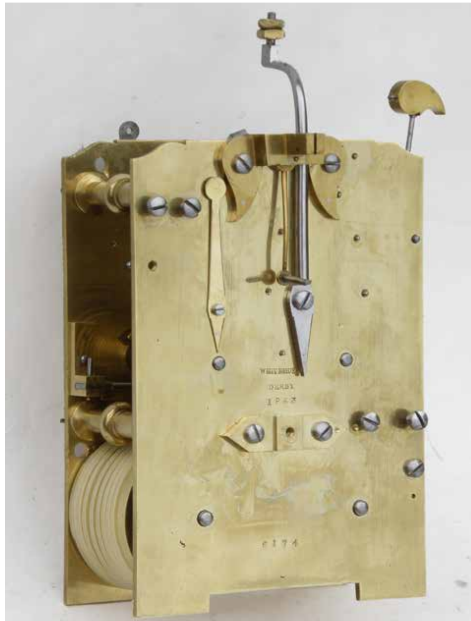
Figure 4. Rear of the movement showing the biasing spring for the strike / silent and the hold-fast for the pendulum.
