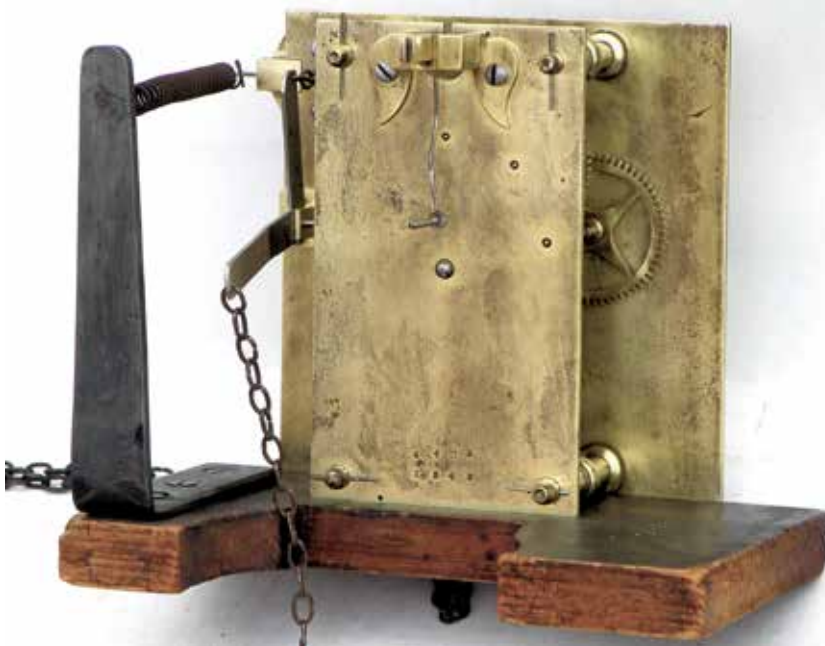
Figure 7. Rear view showing the sturdy iron bracket for the return spring.
