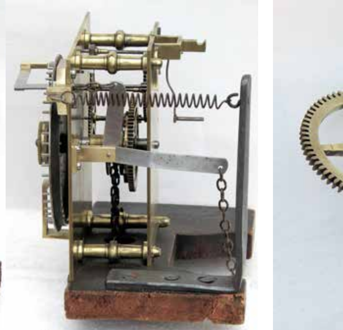
Figure 8. Side view with the lever mechanism to depress the pins.
