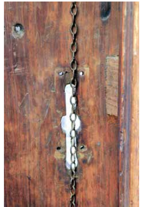
Figure 25. The pull chain exited round a pulley and through a hole in the backboard.
