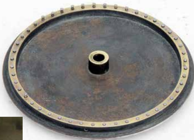
Figure 18. The heavy brass rotating dial with pins through the rim.
