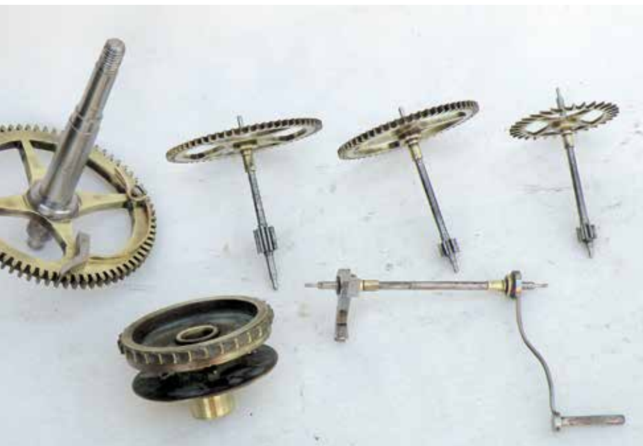
Figure 9. The four wheels, chain pulley with ratchet and anchor pallets.
