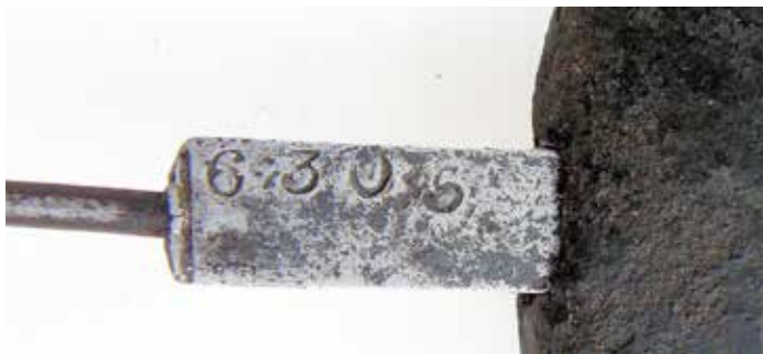
Figure 13. The pendulum flat stamped with a 3 instead of a 4 by mistake.
