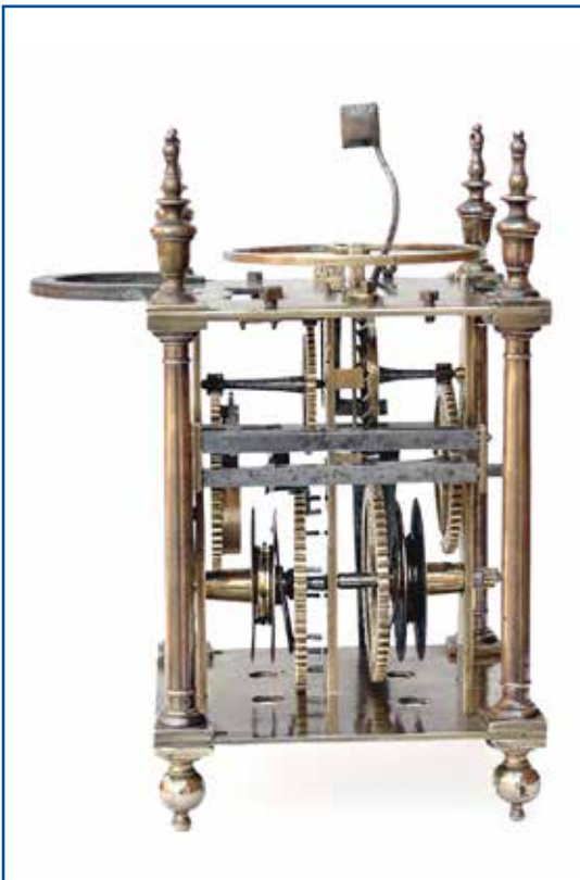
Figure 22 (above left). Front of the movement with an iron hour wheel and a five-leaf pinion-of- report.
