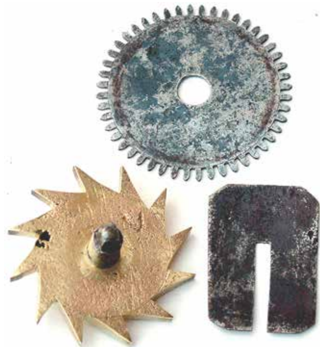
Figure 19. The motionwork, with a solid starwheel and an iron hour wheel.
