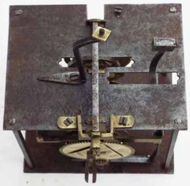
Figure 12. Top of the movement showing the pallet arbor, with no aperture for the fly.
