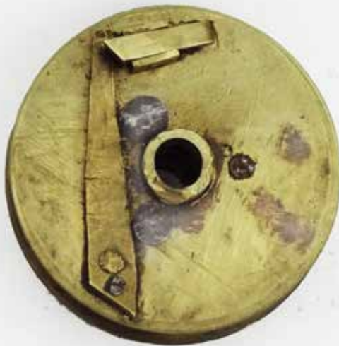
Figure 8 (above). Chain pulley with a spring-loaded pivoted click.
