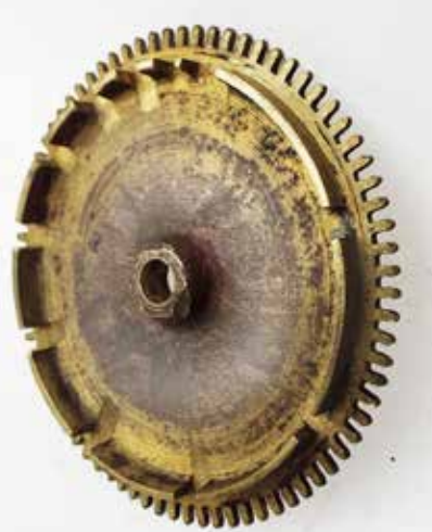
Figure 9. Countwheel with integral slotted ring and gear teeth.
