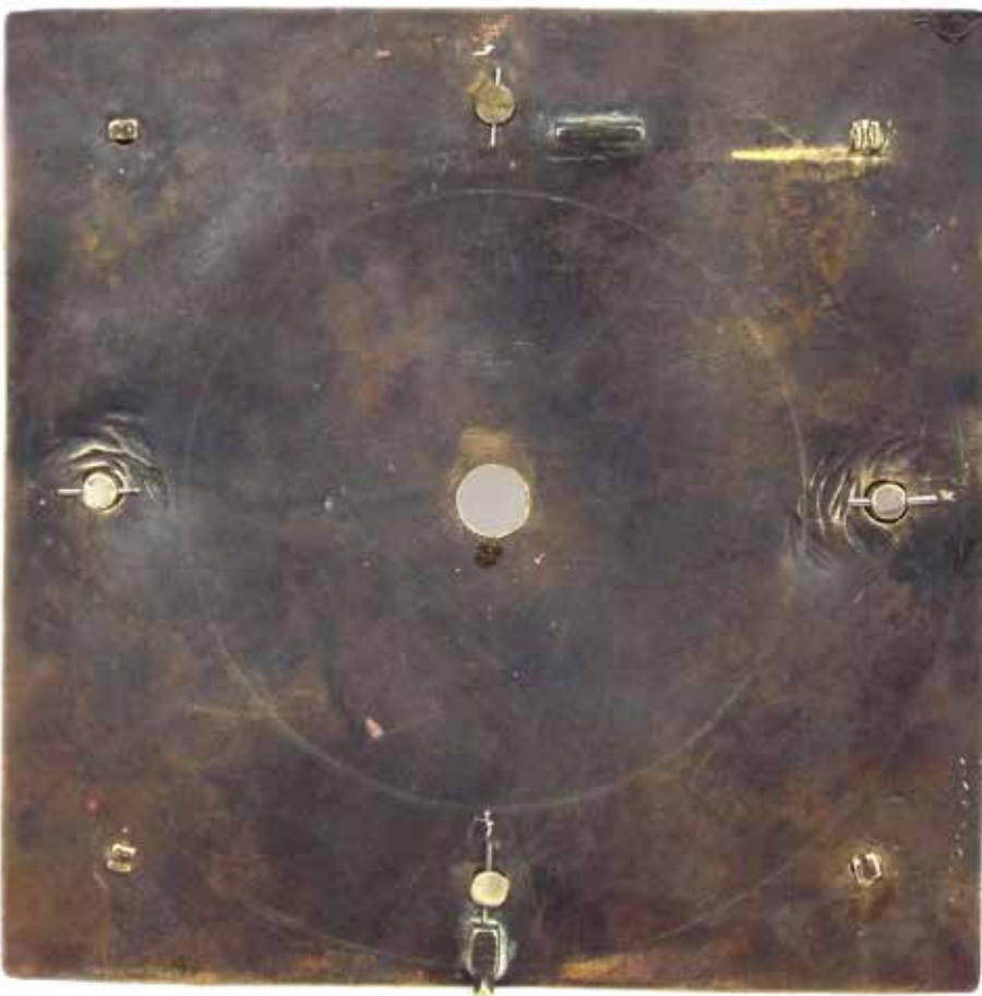
Figure 14. Movement with the hour and minute wheels removed.
