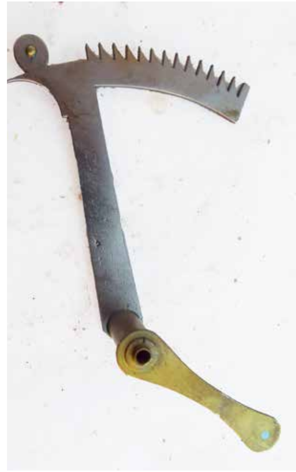
Figure 16. The straightened rack tail.
