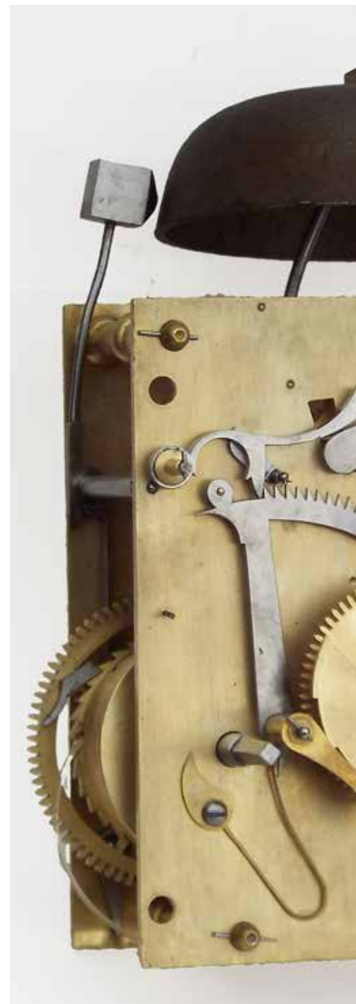
Figure 18. Movement with the moon wheel removed.
