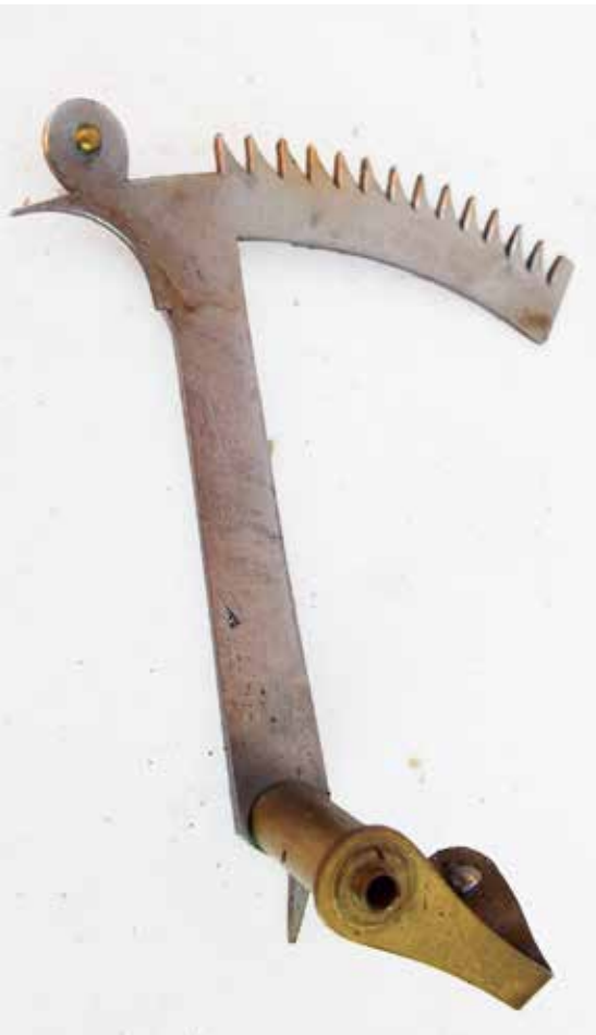
Figures 14 and 15. The damaged rack tail.
