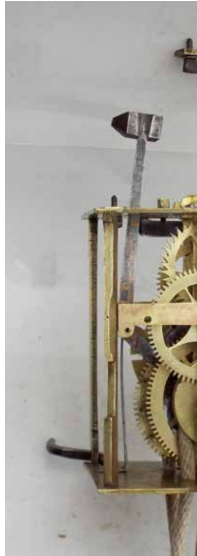
Figure 4. Movement with the hour wheel removed.
