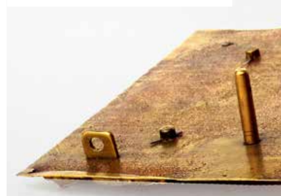
Figure 2. Dial rear showing the original tabs and later dial feet.
