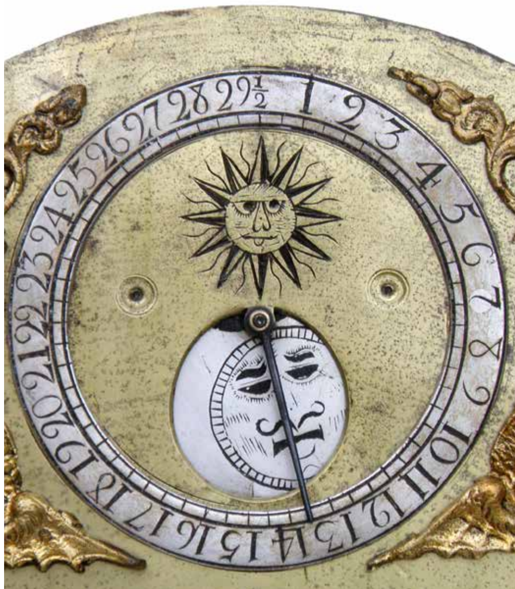
Figure 3. The penny moon and the silvered ring showing one lunation of 29\frac{1}{2} lunar days.
