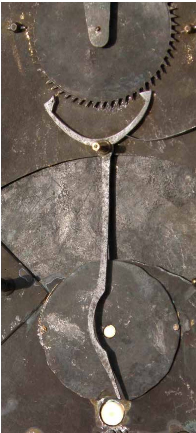
Figure 7 (left). The operating mechanism for the penny moon.
