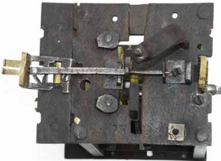
Figure 19. Top of the movement showing the escapement and modified backcock.
