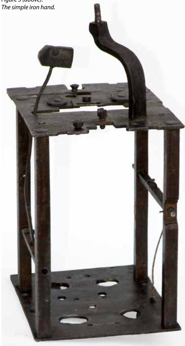
Figure 7 (above). Original iron movement bars and the later brass bar.
