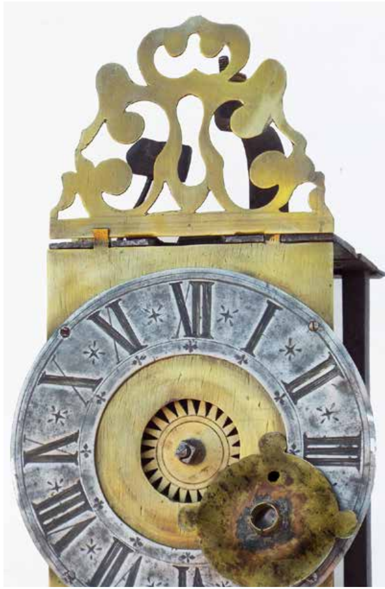
Figure 4. Cut-off pin on the back of the alarm disc and the large central hole in the dial.
