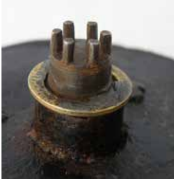
Figure 12 (above). Striking train from a Dutch clock.
