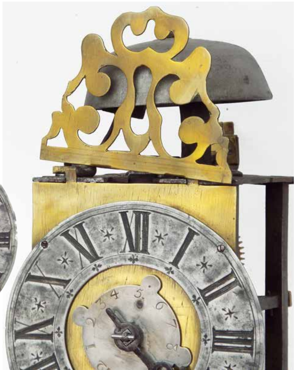
Figure 2. Tabs at the top of the dial held by the thin fret.
