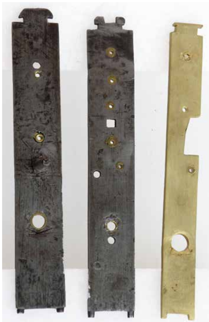
Figure 7 (above). Original iron movement bars and the later brass bar.
