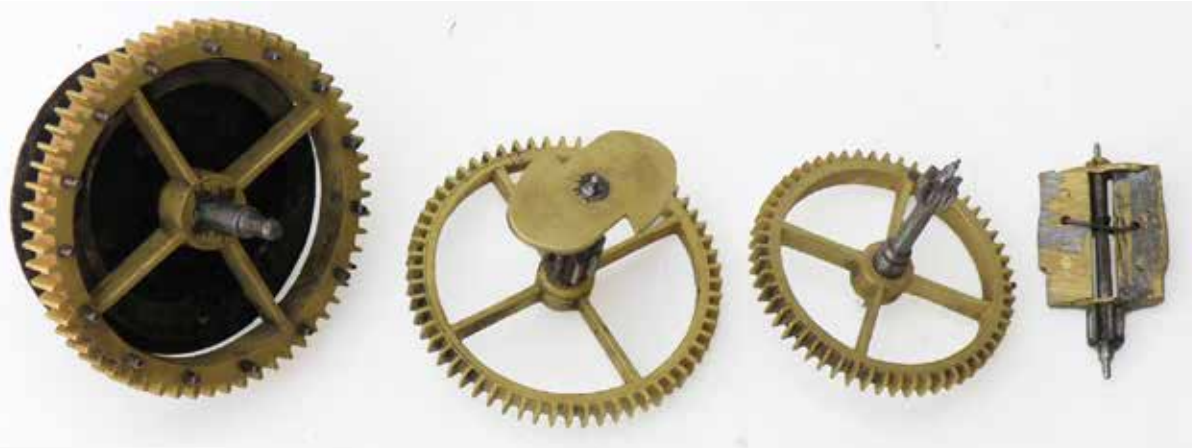
Figure 12 (above). Striking train from a Dutch clock.
