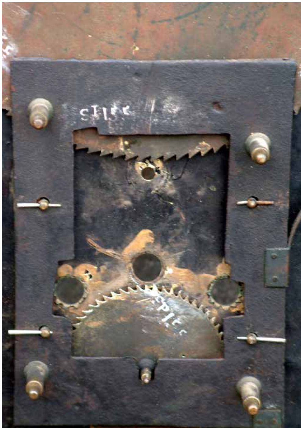
Figure 3. Falseplate, moon and calendar of the Fisher dial with stamped 'SP133'. Photograph by John Robey.
