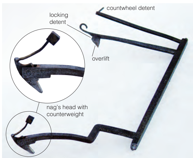
Figure 13. The one-piece arbor for warnless striking using a nag's head.
