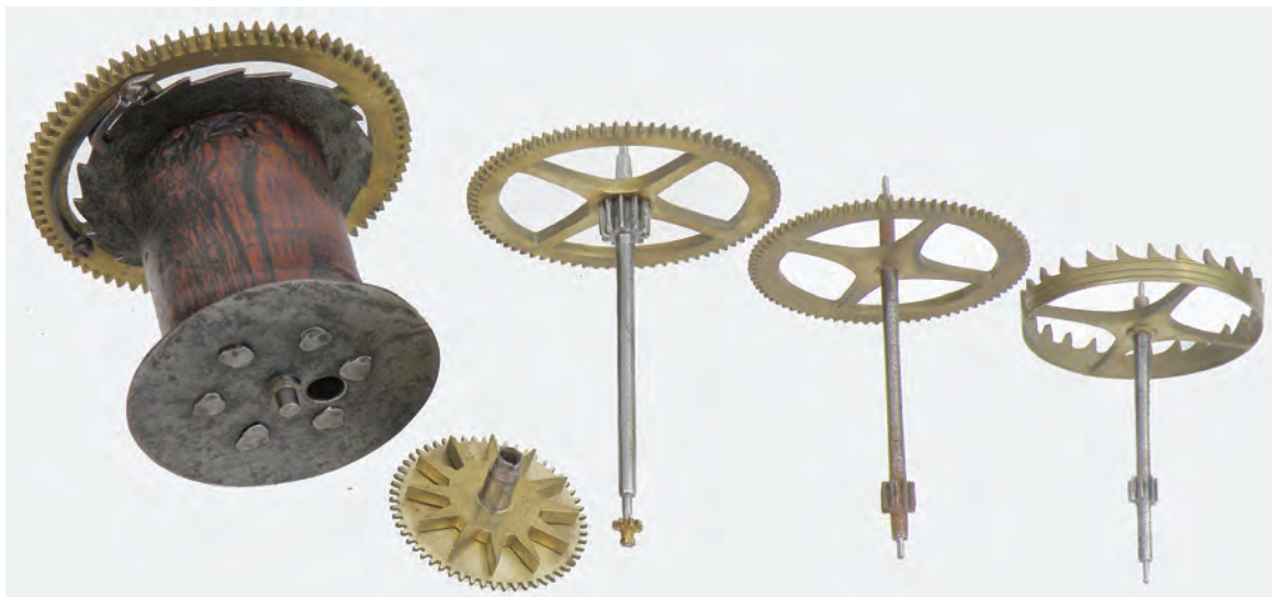
Figure 8. Alternate leaves of the pinion-of-report are of only half height.
