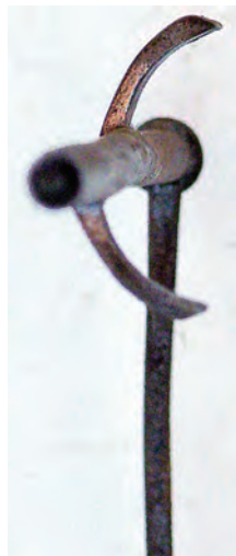
Figure 11. The curved pallets with a very wide angle between them.
