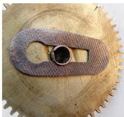
Figure 9. The spring for hand setting made from an old thin file.
