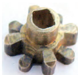
Figure 8. Alternate leaves of the pinion-of-report are of only half height.
