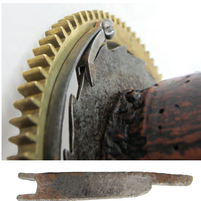
Figure 7. A slot in the click restrains the barrel's sideways movement.
