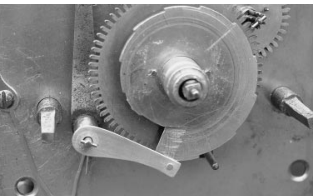
7 The finished rack tail.
