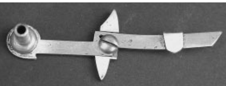
9, 10 The adjustable rack hook of the Cooke clock.
