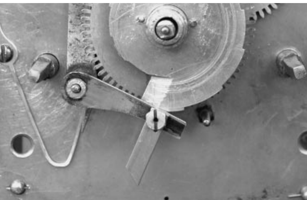
3. 4. Jig for determining the position of the contact pin on the end of the rack tail.
