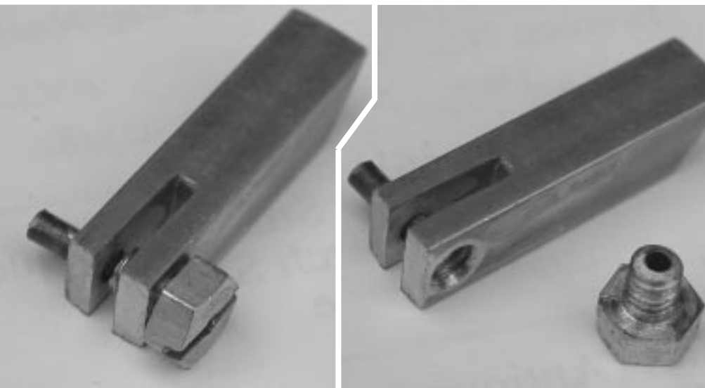
3. 4. Jig for determining the position of the contact pin on the end of the rack tail.
