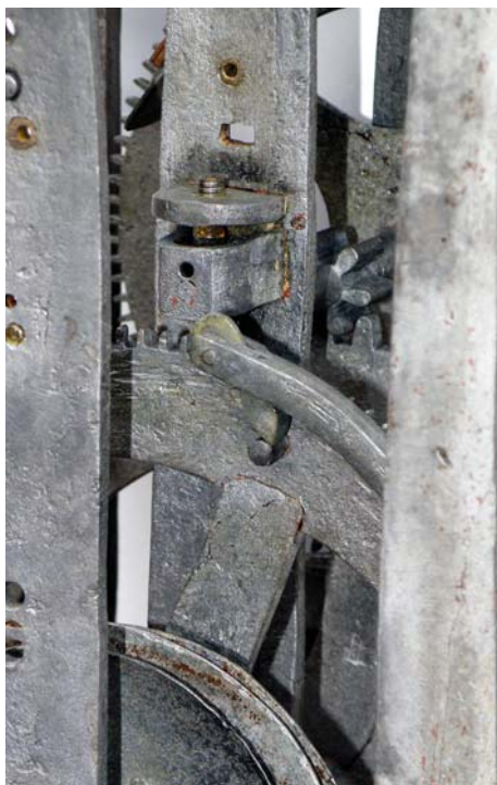
4. A pin on the greatwheel moves the nag's head without raising the lifting piece.
