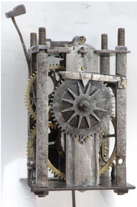
8. A small 30-hour iron wall clock, probably German, with nag's head striking let off by an iron starwheel. The hole in the right-hand pillar is for a missing half-hour passing strike.
