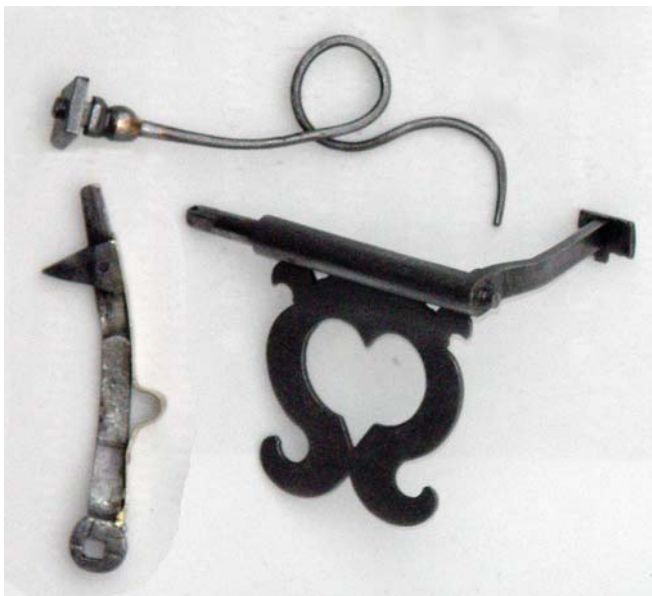
12. The lifting piece and nag's head (left) fit onto the squared end of the arbor which has a shaped trip piece and combined detents. Above is the return spring.
