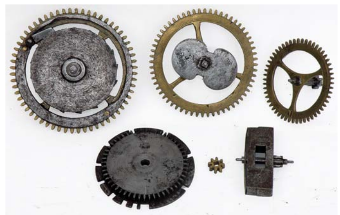
The striking train and countwheel showing the double heart on the arbor of the second wheel.
