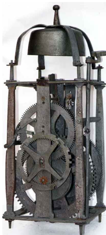
2. Rear view of a large iron clock about 1600-50 with only two wheels in each train (later escapement and wheels not shown). On the left is the striking arbor with the countwheel detent, overlift lever and locking detent (just visible behind the locking wheel).
