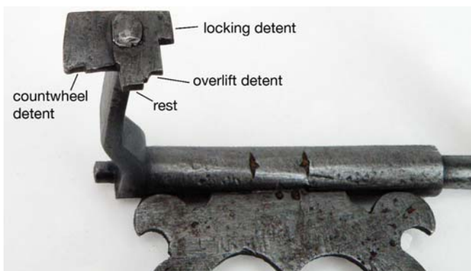
13. Details of the combined locking, overlift and countwheel detents.
