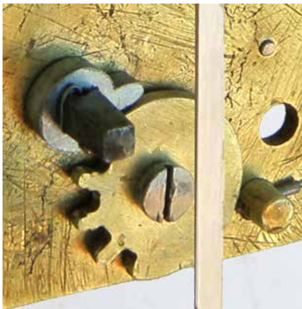
Figure 21. The stopwork shown with the mainspring in the fully wound position
