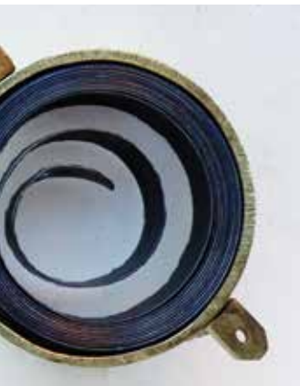
Figure 18 (above). The barrel wheel with its ratchet and click and the standing barrel.
