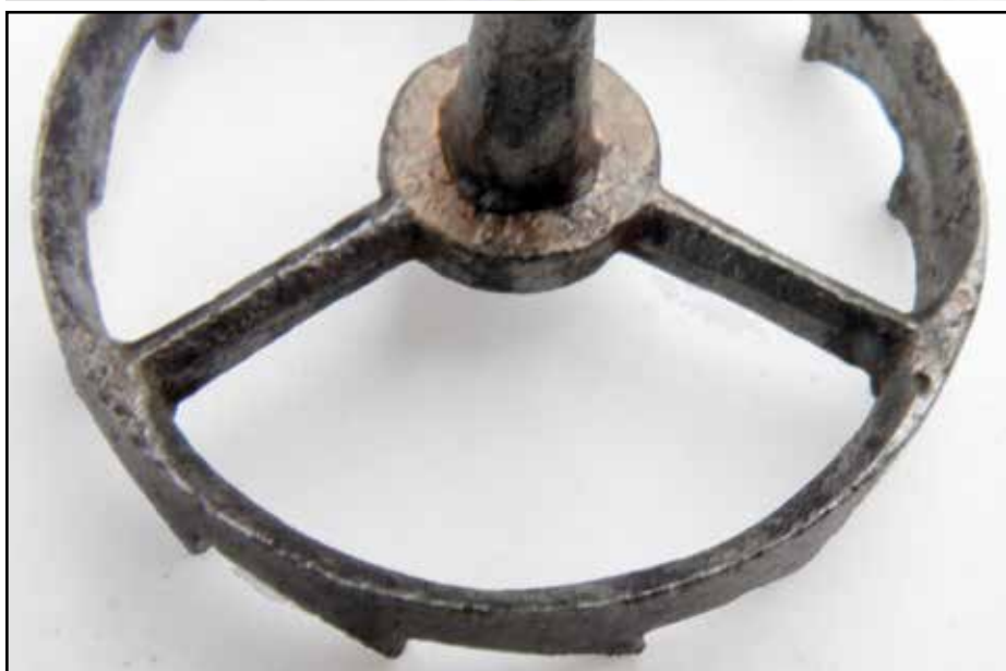
Figure 12. Marking-out dots on the teeth of the going great wheel. Note the forged join between the crossing and the rim.
