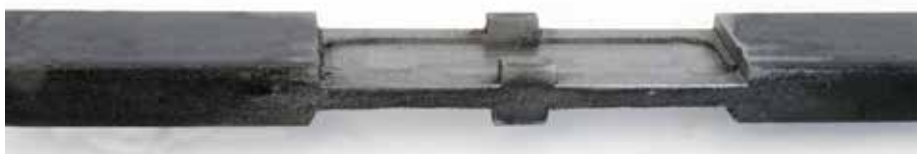
Figure 19. First stage in making a replacement fly.
