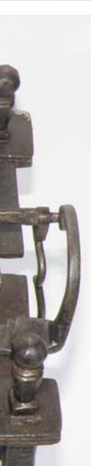
Figure 9. Movement from the right showing the long locking arbor and the short warning arbor.
