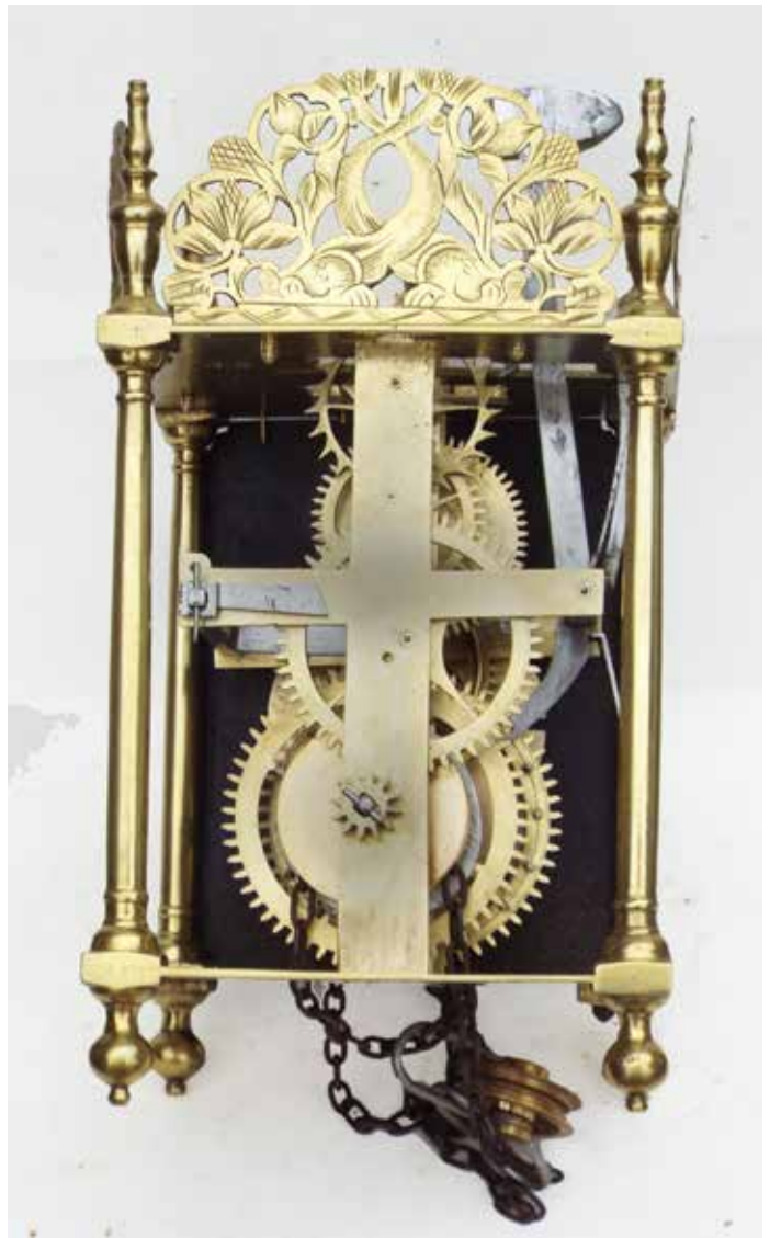
Figure 3. Movement with the hour wheel removed.
