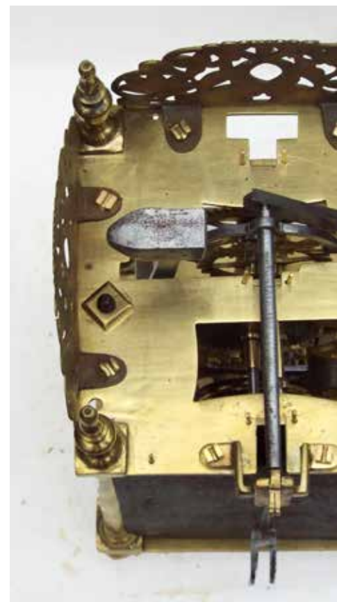
Figure 7. The top plate and the anchor escapement.
