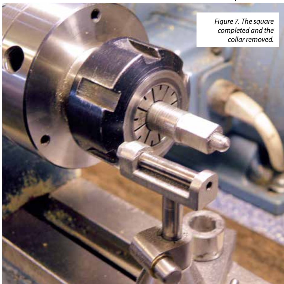
Figure 8. The finished arbor with a small square to take the count-wheel pinion.
