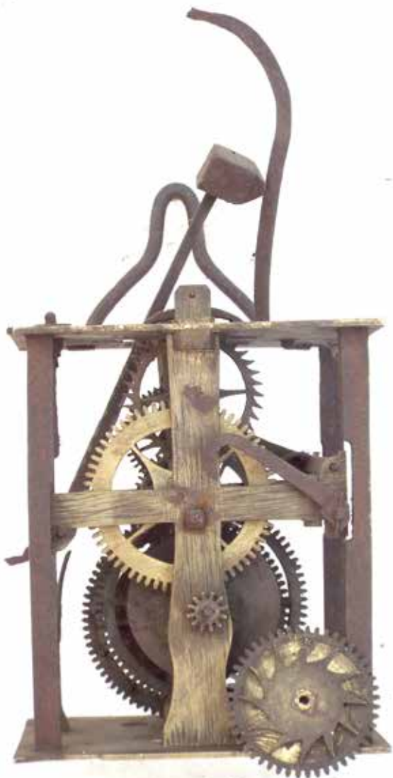
Figure 6. The movement with the hour wheel removed.
