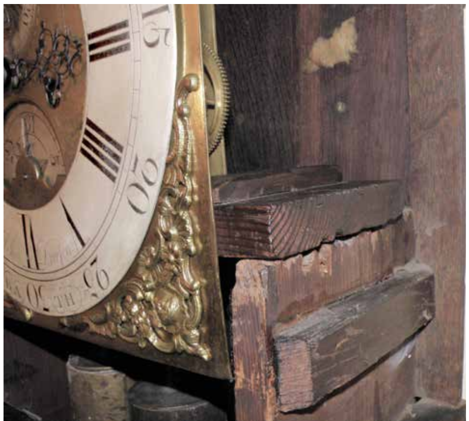
Figure 14. There is no packing between the seatboard and the cheeks.
