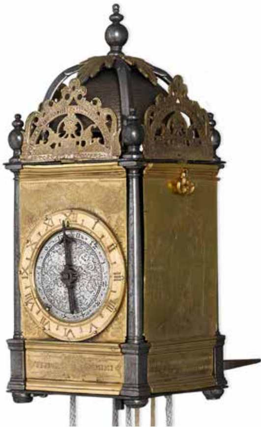
Figure 7. Weight-driven Flemish Renaissance clock, about 1580, with an iron frame.
