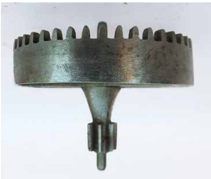
Figure 17. The contrate wheel with a steeply tapered arbor.
