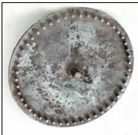
Figure 18 (top left). The contrate wheel with three crossings.
