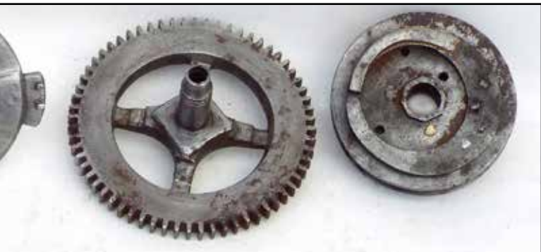
Figure 14. The going greatwheel assembly; left: ribotta pins and tabs for setting the hand; centre: the greatwheel; right: rope pulley and spring click.
