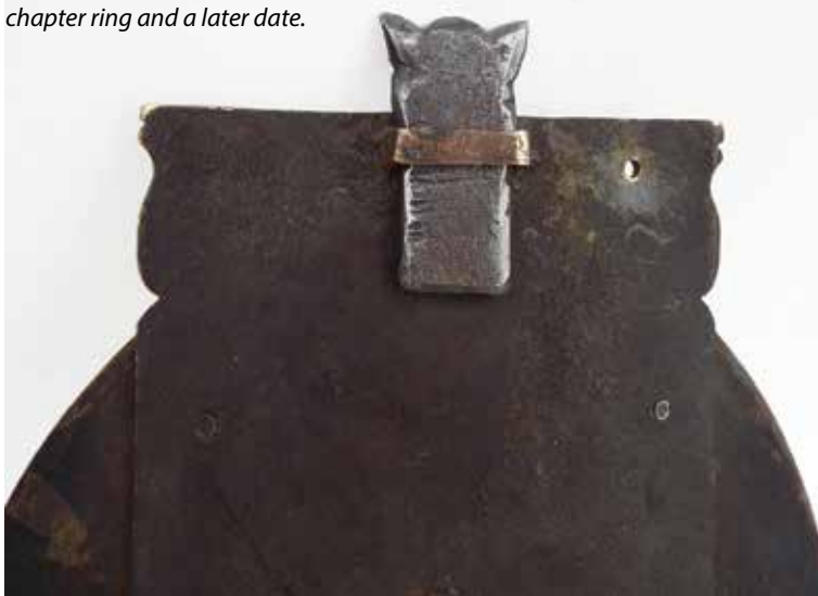
Figure 5. Wedge and staple for holding the top of the dial.
