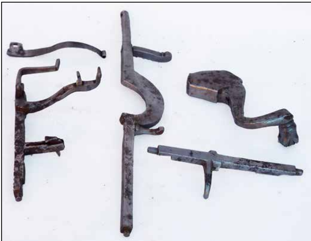
Figure 25 (far left). To left: auxiliary hammer spring; left: strike-work arbor with nag's head; centre: vertical hammer shaft; top right: hammer head; bottom right: horizontal arbor with hammer tail.
