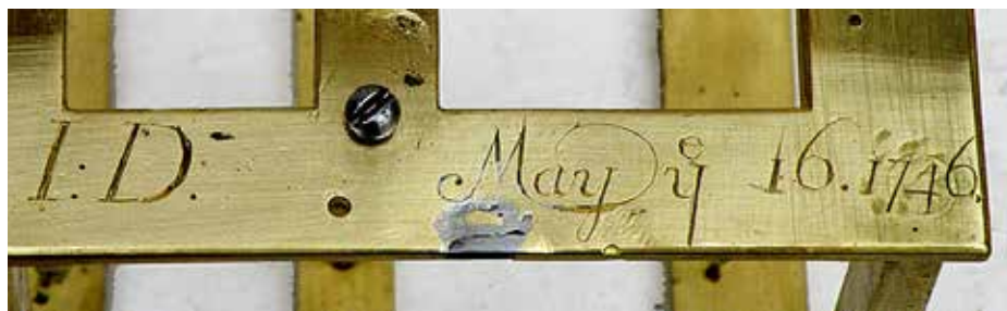
Figure 25. Joseph Donisthorpe's initials and date engraved on the top plate. Note the iron insert where the hammer shaft stops.
