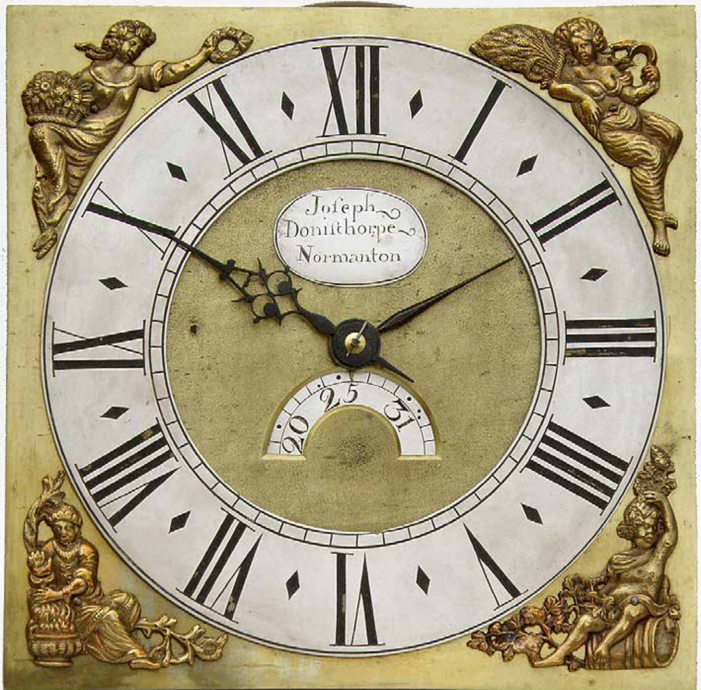
Figure 19. The dial of Clock 2, similar to Clock 1 but with a calendar and an alarm hand.
