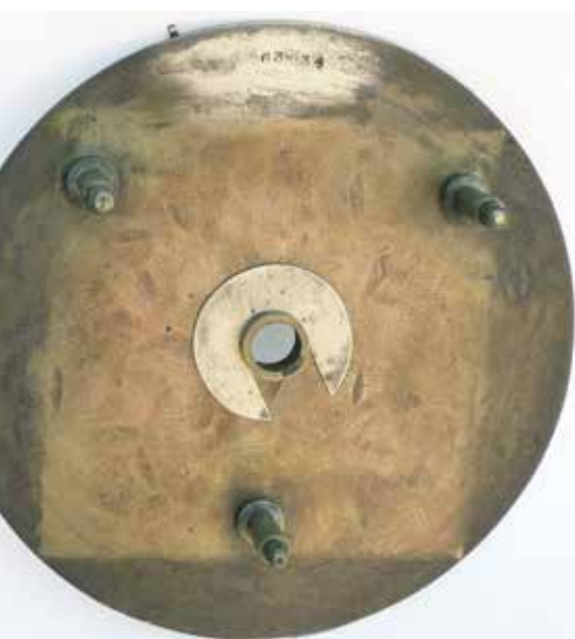
Figure 37 (below). Dial rear with the boss of the alarm hand held by the slip washer.
