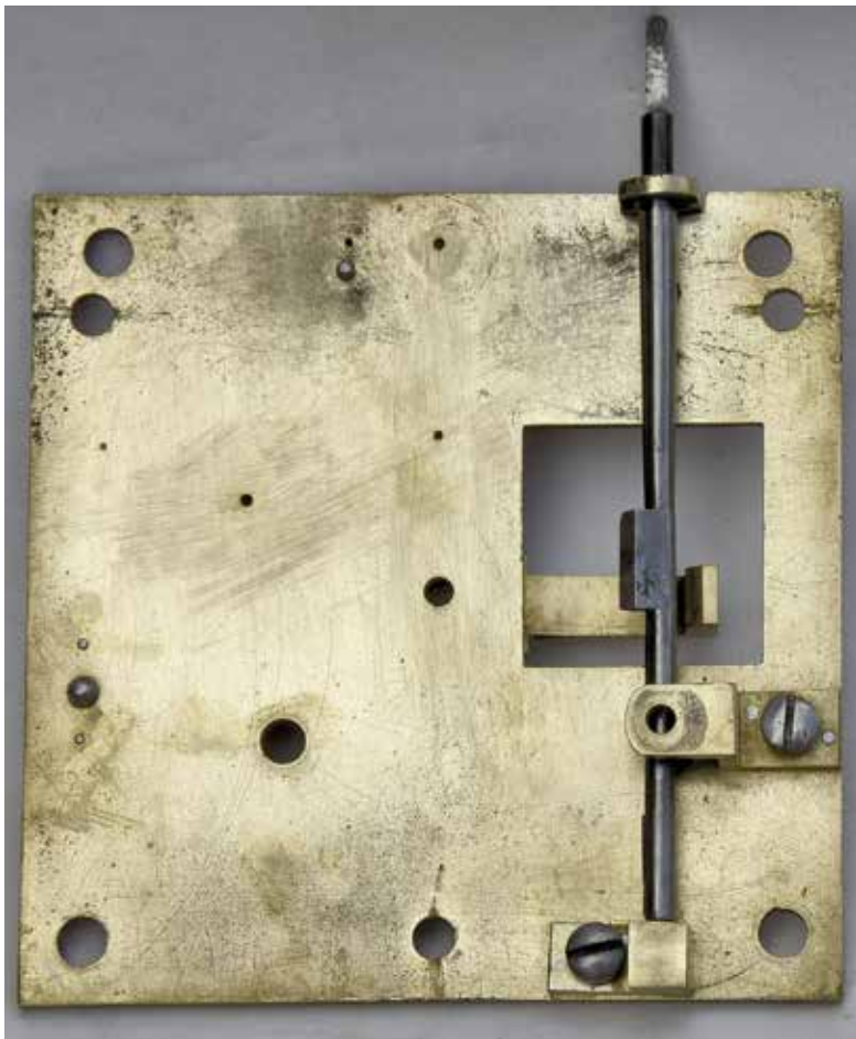
Figure 33 (above left). Rear of the front plate with the alarm verge.
