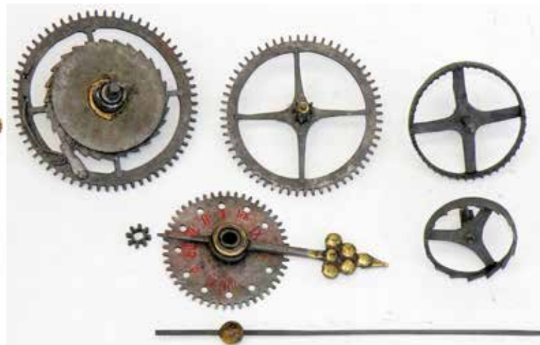
Figure 7. The going train, verge pallets and pendulum.
