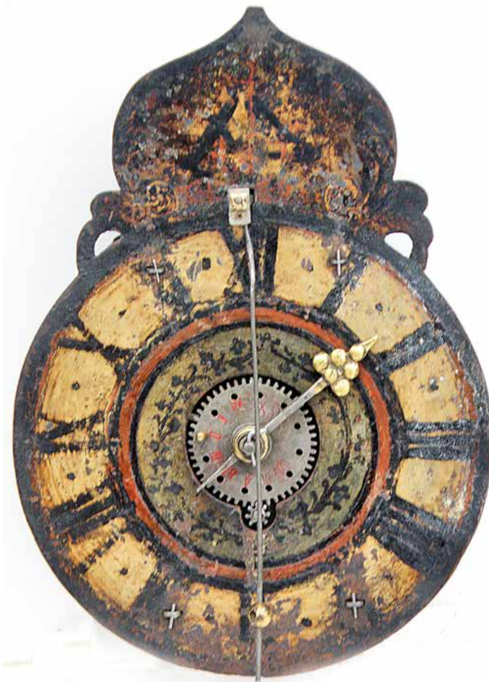
Figure 1. Late seventeenth-century 30-hour iron timepiece alarm with a single hand.
