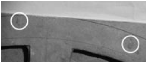
Fig. 10. Rear of a dial by John Dumvile of Alderley, Cheshire, showing two impressions from a fault on a hammer head.
