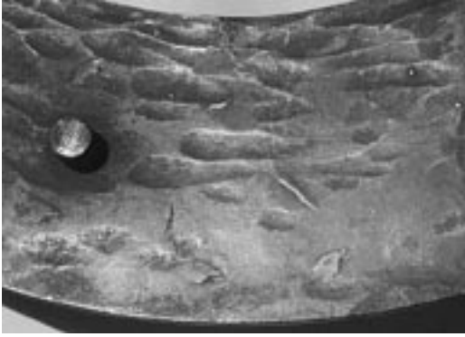
Fig. 8. The same hammer mark on the rear of the chapter ring. As well as the flat-faced hammer with its fault, the chapter ring has also been heavily beaten with a narrower peening hammer.
