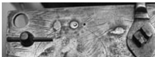
Fig. 3. Detail of two of the marks made by a hammer with a chip or other fault on its working face, on the top left-hand corner of the movement.
