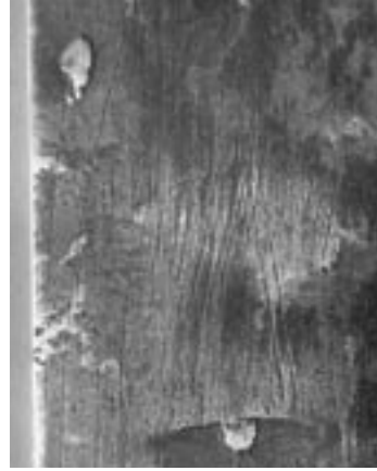
Fig. 6. Detail of hammer marks near the left-hand edge of the dial.
