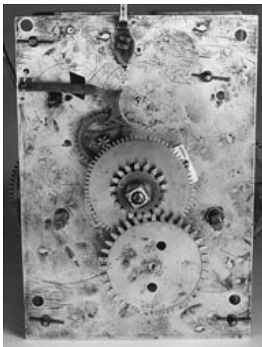
Fig. 2. Front of the movement with hammer marks clearly visible.
