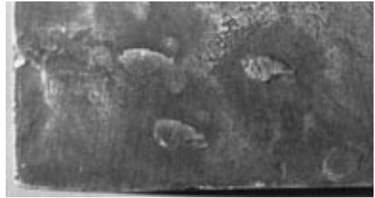
Fig. 7. A group of hammer marks at the bottom left-hand corner of the dial.
