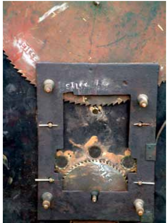
Fig. 3. Rear of the Fisher dial with SP155 stamped on the falseplate, calendar and on the moon, where P and 1 overlap to appear as H.
