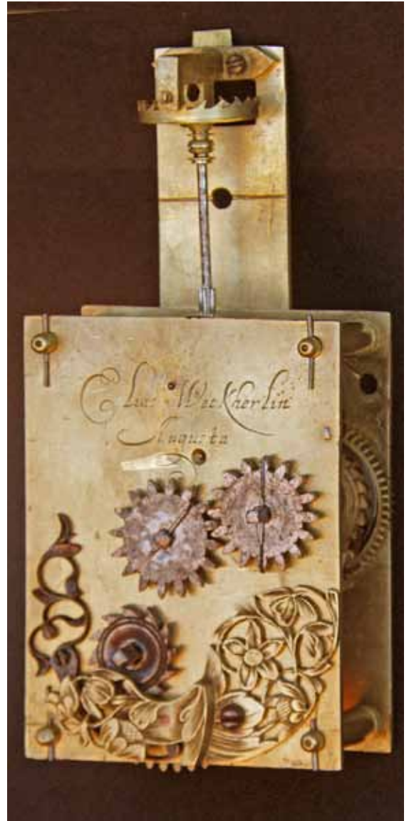
Movement from the rear. Note the two iron wheels to connect the winding square with the rear of the fusee. Decoratively engraved and fretted brass set-up click. The crownwheel has a long turned and finned collet.
