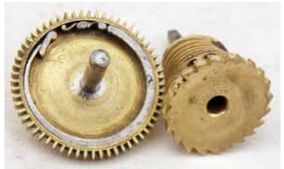
Above: detail of the verge-and-crownwheel escapement. Below: the fusee with its exposed click and spring.
