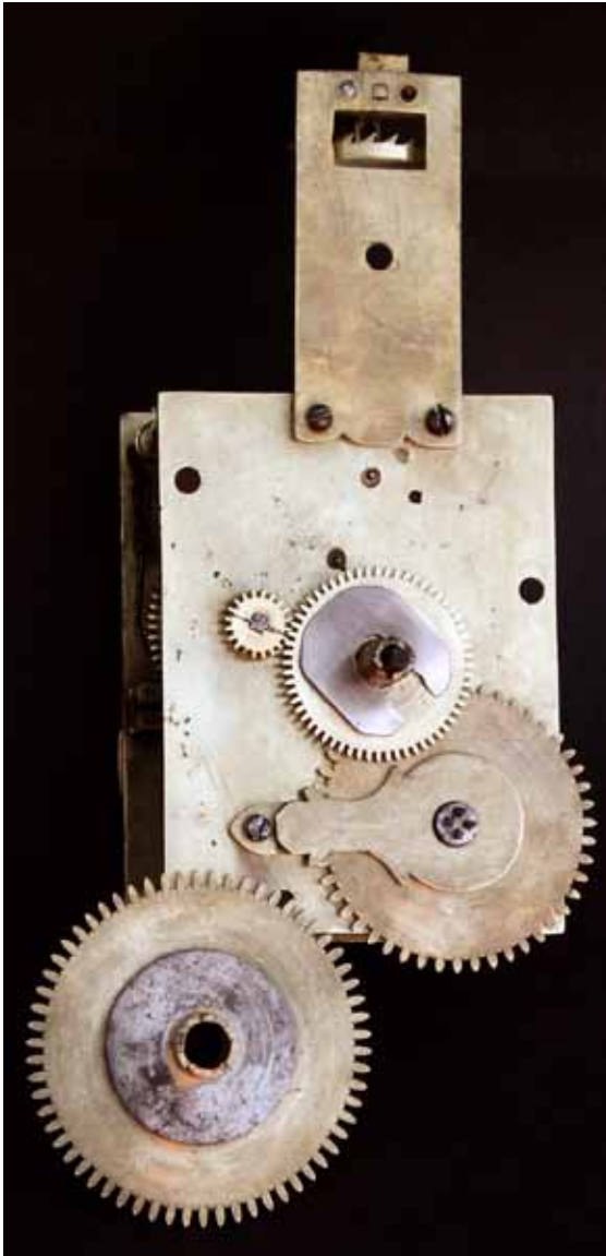
Movement from the front with the calendar wheel removed. The crownwheel pivots in a vertical extension screwed to the front plate.
