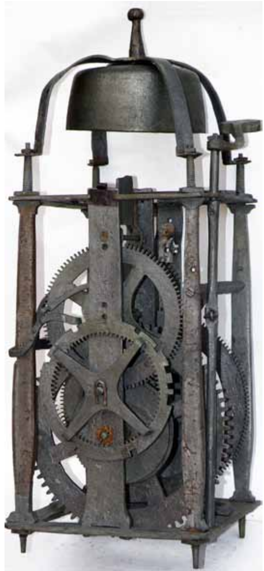
Fig. 4. Rear view showing the countwheel with slots on the outer edge, gear teeth on the inner edge and offset crossings. Only two wheels and a fly in the striking train.
