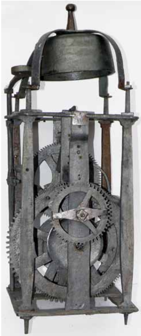
Fig. 3. Front of the all-iron movement with just the original wheels and the later dial wheel. Note the slim baluster-shaped pillars and the pin on the going greatwheel to let off the strike.
