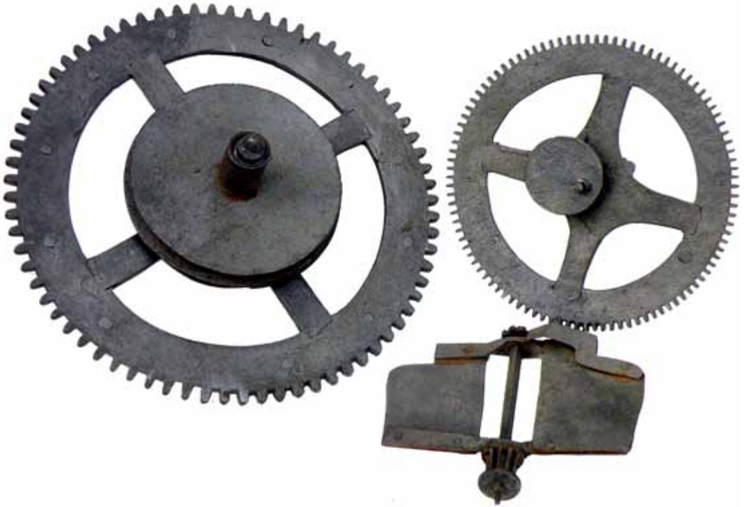
Fig. 9. The striking train of just two wheels and a fly. Note the later off-centre disc on the second arbor to provide overlift. The lantern pinion on the fly arbor is a later repair.
