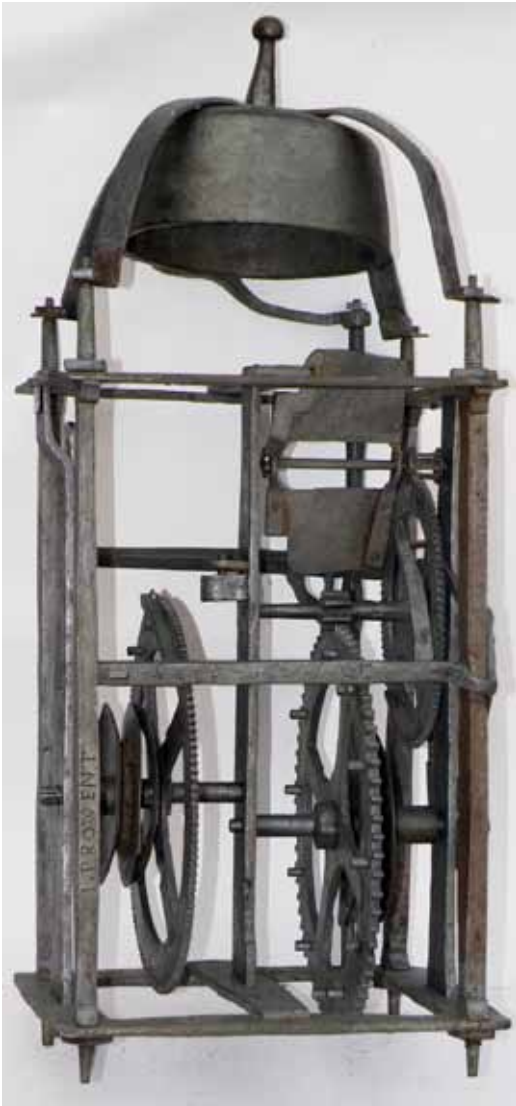
Fig. 5. Right-hand side with the single-arbor strikework. The bridge for the crownwheel of the original balance escapement survives on the central movement bar. Above it is the bottom block with an adjusting screw for the crownwheel of the replacement short pendulum escapement. The name 'I, PROWENT' can be seen on the left-hand pillar.
