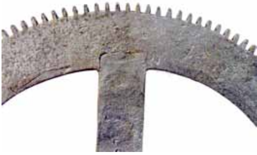
Fig. 7. The going greatwheel with a correctly formed join of the crossings to the rim.
