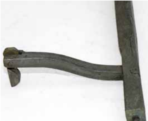
Fig. 11. Striking arbor with the nag's head and locking detent. The later overlift arm is riveted to the countwheel detent. The vertical hammer is in the foreground, with the hammer tail on its own arbor above it.
