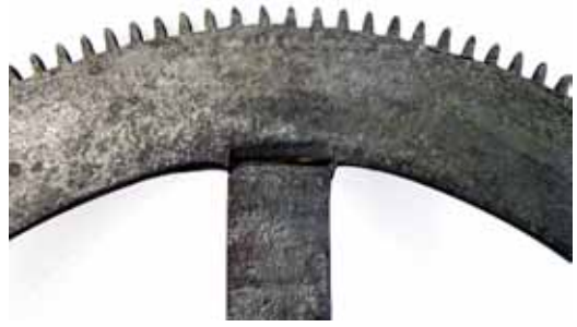
Fig. 8. A join with part broken off showing the end of the crossing fitting into V-notches filed into the inner edge of the rim.
