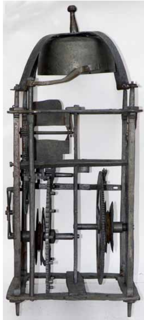
Fig. 6. Left-hand side showing the hammer head on the outside of the bell and the vertical shaft. The missing hammer spring and hammer stop ('counter') have since been restored. Note the large sheet-iron fly.
