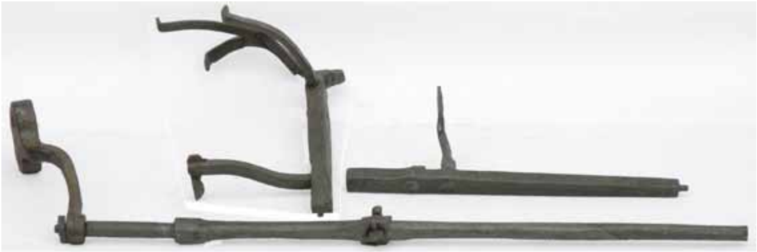
Fig. 11. Striking arbor with the nag's head and locking detent. The later overlift arm is riveted to the countwheel detent. The vertical hammer is in the foreground, with the hammer tail on its own arbor above it.
