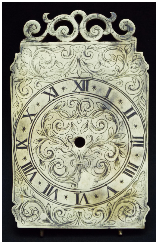
Fig. 11. The single-sheet brass dial with an integral fret.
