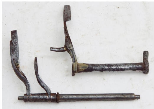
Fig. 23. The warning/lifting detents (top) sit over the locking/countwheel detens (below).
