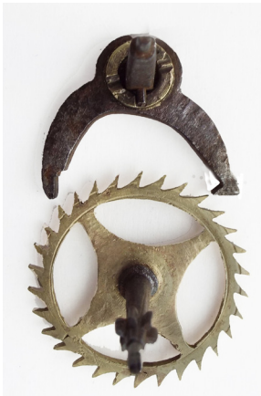
Fig. 24. The very early anchor escapement, added about 1675-1700.
