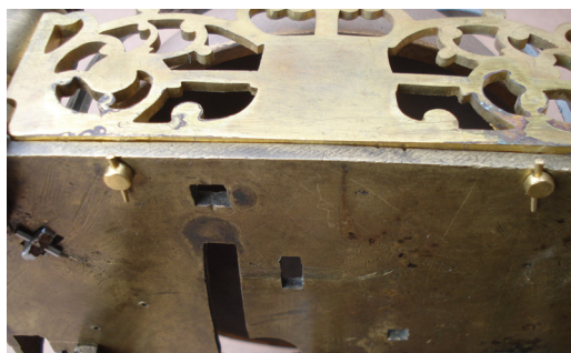
Fig. 32. The unique pinned feet to hold the frets. (Private collection)
