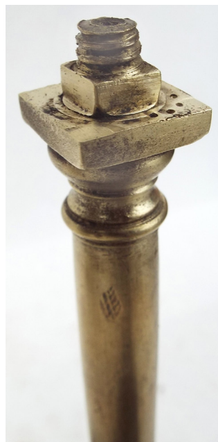
Fig. 17. Pillar with an integral screw and a square boss that fits into the bottom plate.
