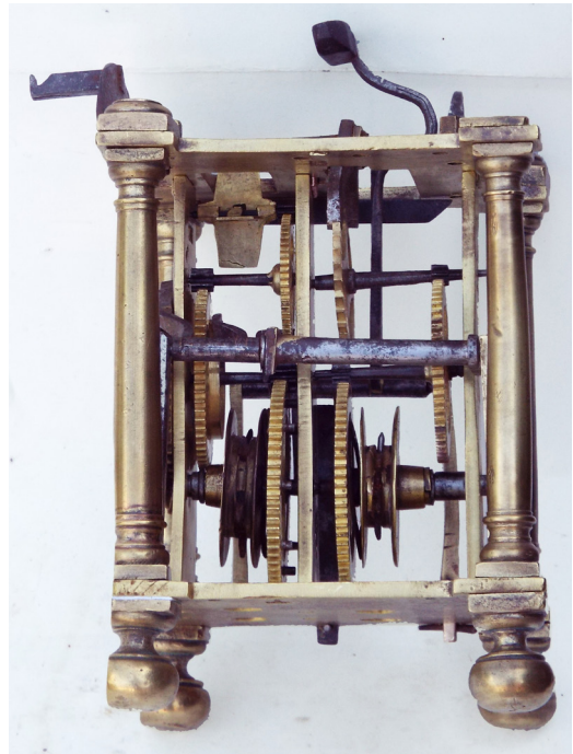
Figs 12-15. The movement after cleaning. There is no hoop or spikes for hanging on a wall.
