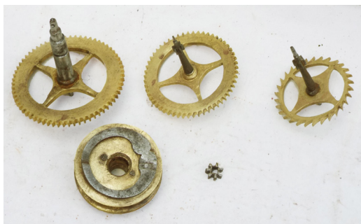
Fig. 18. The going train with a later escapewheel and pinion-of-report.
