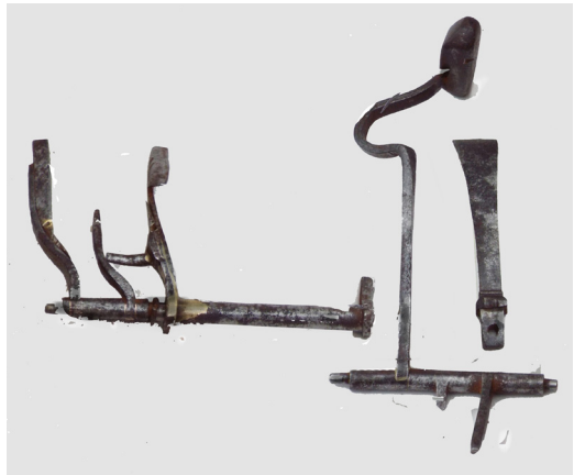
Fig. 22. The concentric strike-work (left), hammer and hammer spring.
