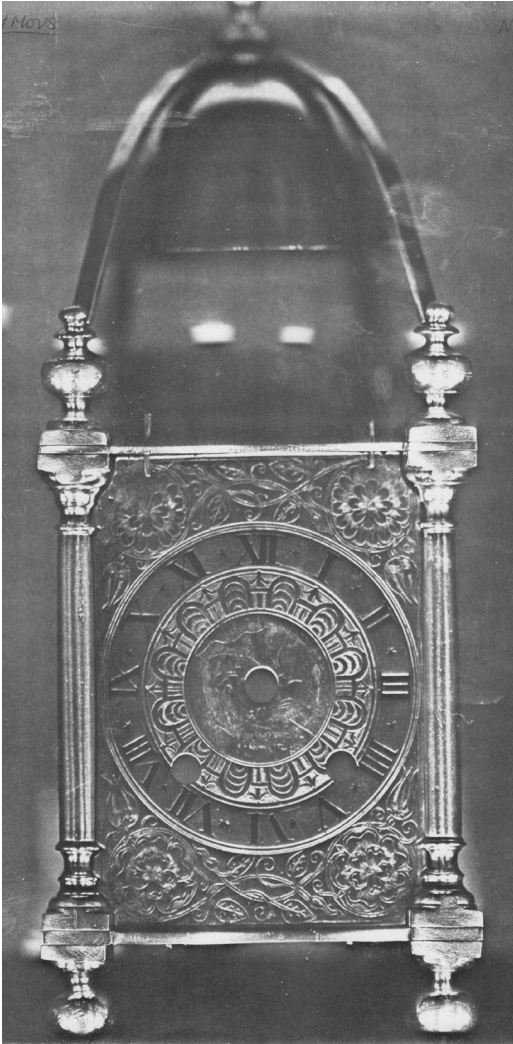
Fig. 26. The frame of an early clock from the Harvey workshop with a single-sheet dial. (Peter Harding courtesy of David Todd)
