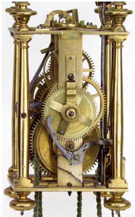
Fig. 5. Movement from the front showing the alarm let-off lever.
