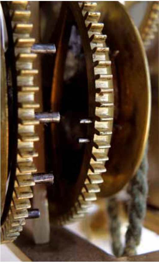
Fig. 9. One of the two sets of double pins on the going greatwheel to provide ribotta .
