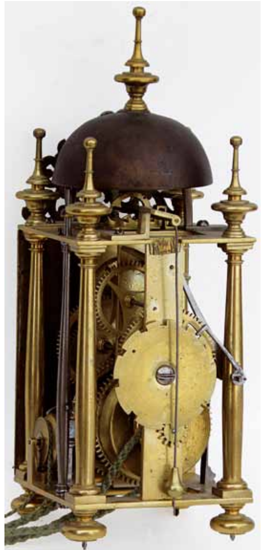
Fig. 2. Rear view showing the countwheel for double striking 1-6 hours.
