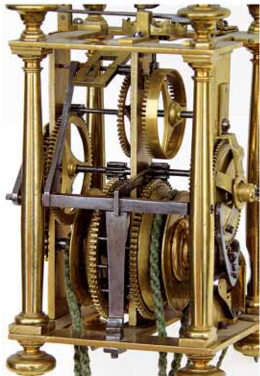
Fig. 7 The left-hand side showing the single strikework arbor.
