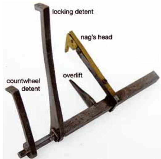
Fig. 10. The strikework arbor.
