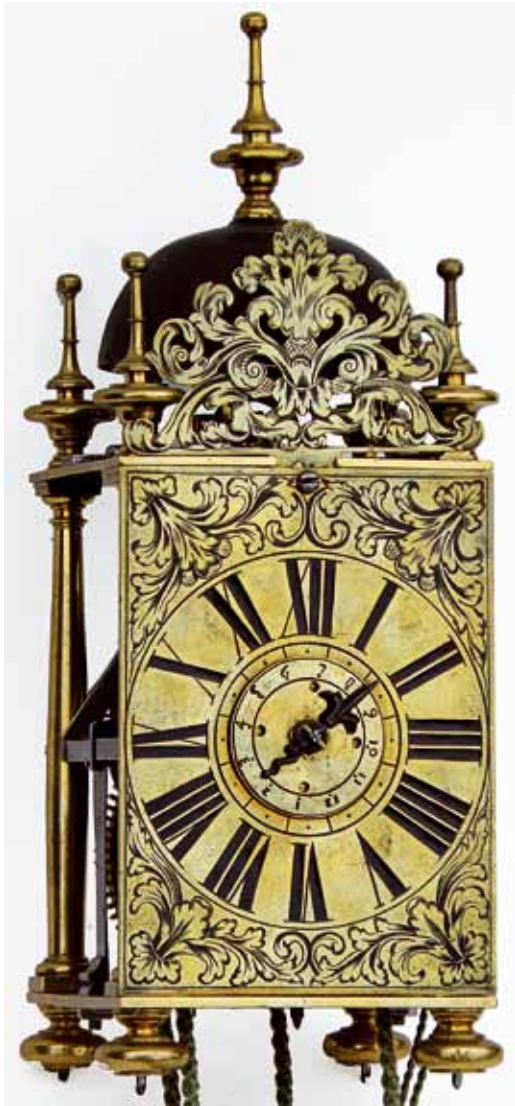
Fig. 1. Small Italian lantern clock with a single-sheet brass dial.
