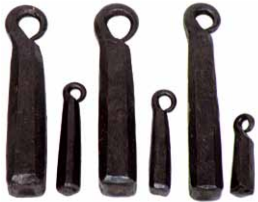
Fig. 4. The iron weights and counterweights with forged eyes.
